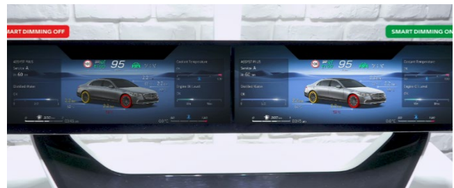
Figure 4: left, how today's display looks in a sunny environment without "perceptual adaptation", Right, cutting-edge perceptual processed content matching the environmental lighting conditions. The environment is measured at 15K lux.
