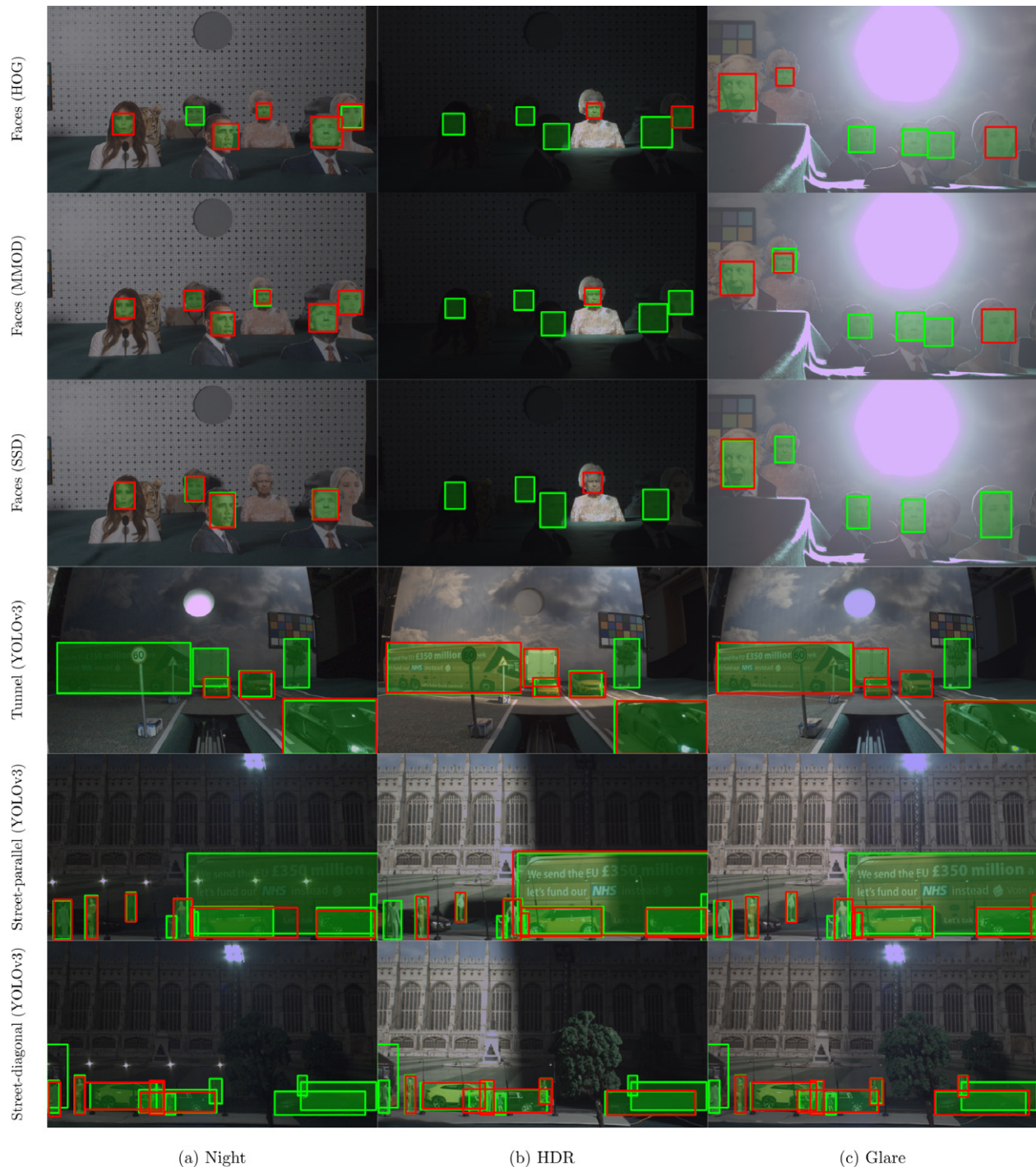
Figure 6. Bounding boxes for several face and object detection methods (rows) for three adversarial illumination conditions (columns), each \gamma encoded (with \gamma = 2.2 ). Faces and objects detected by the various methods for the reference uniform illumination condition are shown as shaded green rectangles, while the results of the tested methods for other illumination conditions are shown as red rectangles.
