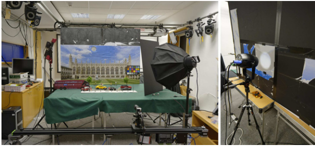
Figure 1. The Street scene along with the capture and setup. Controllable lights are present on either side of the scene to simulate various lighting conditions. The right image shows the spotlight behind the scene, which shines through the diffuser and serves as a source of glare.
