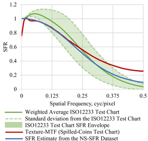
**Figure 4.** This graph shows the vertical system e-SFR estimation from the iPhone7 database. This data is compared to the vertical e-SFR envelope measured from an ISO 12233 test chart and the texture-MTF calculated from the spilled-coins test chart.
