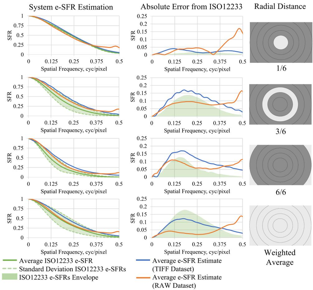
**Figure 3.** The vertical system e-SFR estimation for three radial distances out of six and a weighted mean of all six radial distances. The first column contains the estimated e-SFR in relation to the ISO12233 e-SFR. The second column contains the absolute error of these estimated system e-SFRs. The third column contains a visual representation of the radial distance the data belongs to.
