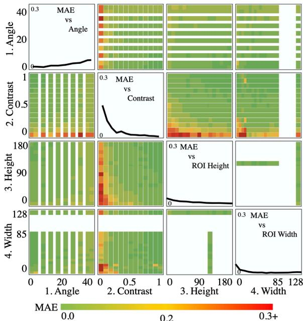
**Figure 1.** Matrix illustrating the variance introduced to the slanted-edge e-SFR measurement when changing edge angle, edge contrast, ROI height and width. The diagonal of the matrix plots the MAE introduced by each SFR parameter.
