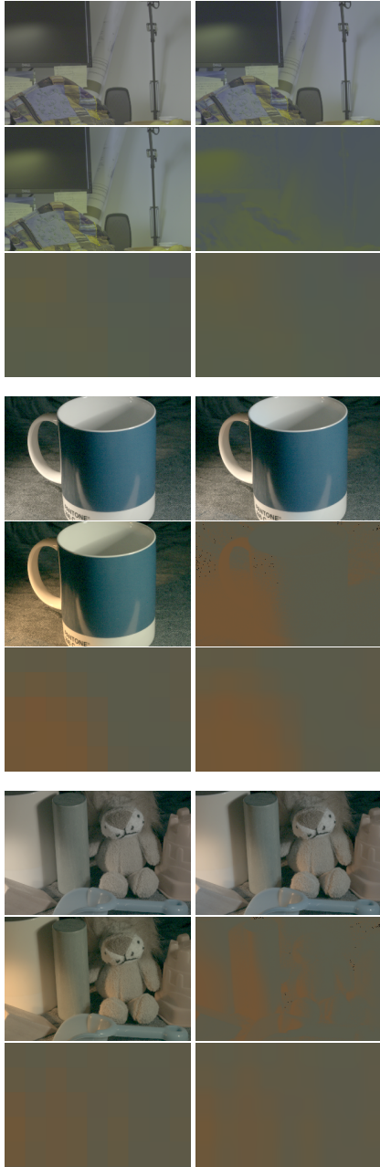
Figure 3. Input data and results of MEM CNN for three scenes from the MIMO dataset. From top to bottom, left to right: image restored with ground-truth, image restored with estimate map, input image, ground-truth image, estimate map, filtered estimate map. The scenes images have the gamma correction applied for visualisation purposes.
