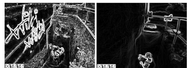
**Figure 9.** Extracting contours from RGB-IR pairs: It is clear that there is much more contrast on the RGB image (on the left). Such samples can be found in our dataset resulting in poor registration based on contours.
