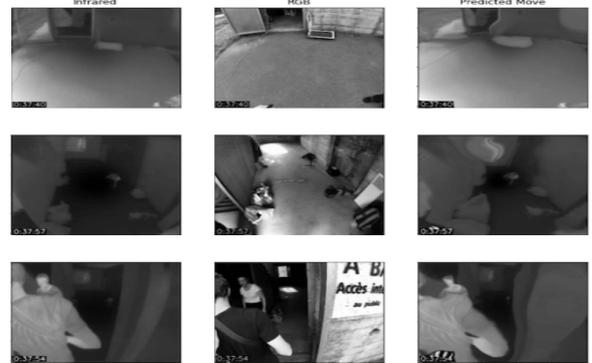
**Figure 2.** Applying the state-of-the-art VoxelMorph model directly on our IR-RGB pairs performs poorly on the challenging scenes in our dataset. We employed a segmentation procedure to tackle this problem leveraging the IR camera's response based on temperature.
