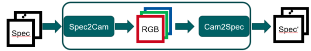
Figure 1: Autoencoder like setup for a joint optimization of a camera response and the spectral reconstruction.
