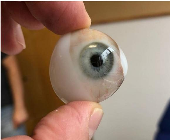
**Figure 1.** 3D printed partly-textured artificial eye. Model was printed with Cuttlefish® [1] on a Stratasys J750 3D printer.
