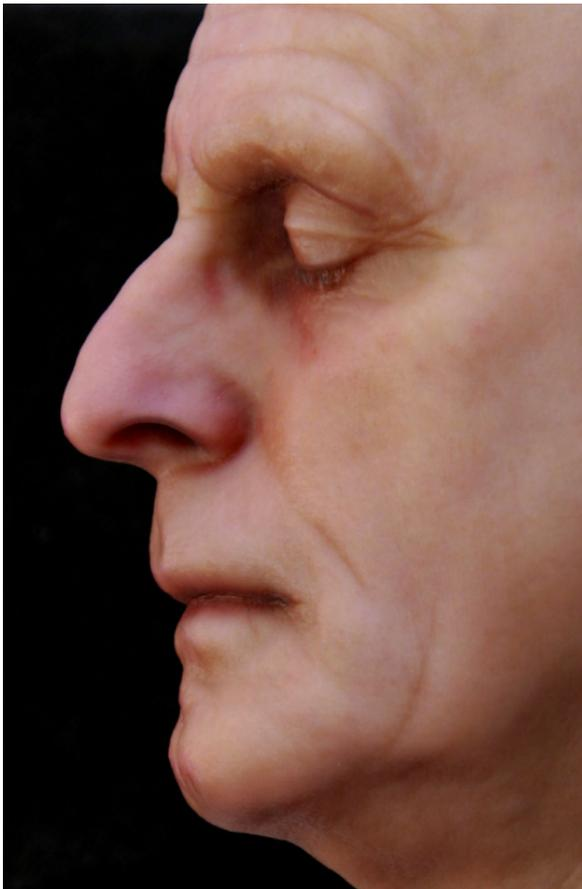
**Figure 4.** 3D printed head model possessing color and translucency of human skin. Model was printed with Cuttlefish® [1] on a Stratasys J750 3D printer.
