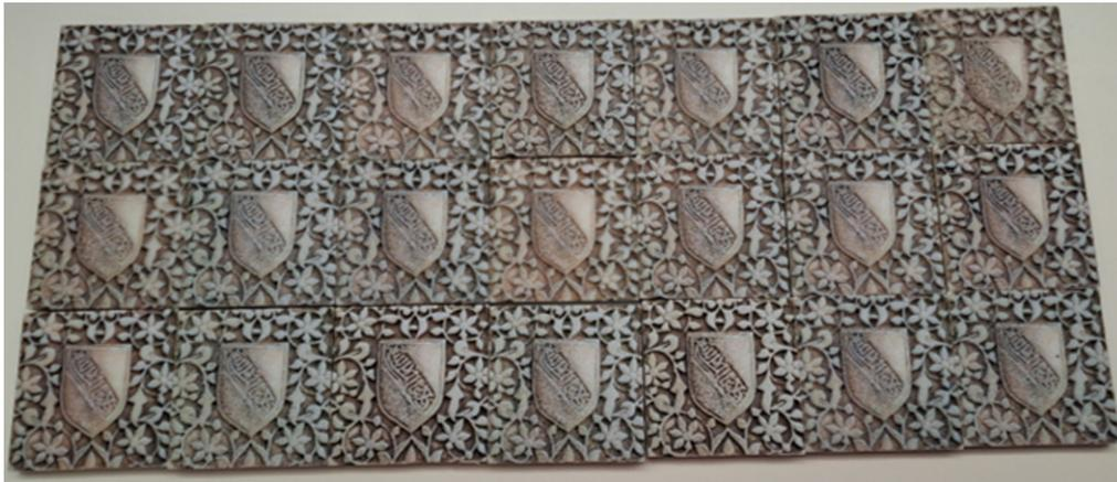
**Figure 5.** Twenty-one printed samples of the Alhambra set. The change in appearance attributes (such as sharpness, elevation, roughness, and color) resulting from variations in surface structure is visible.
