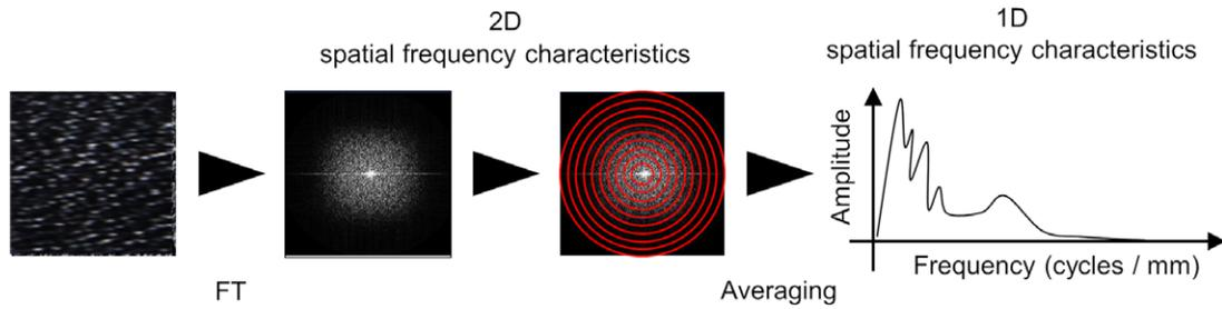
Figure 5. Calculation of characteristics of spatial frequency of the  $L^*$  image.
