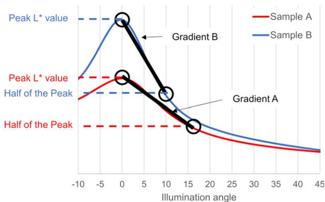
Figure 7. Example of method to calculate the value of the  $L^*$  gradient.
