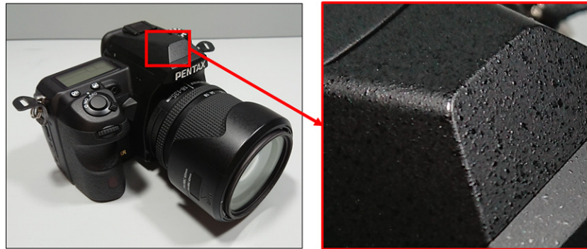
Figure 1. Exterior of a digital single-lens reflex camera and magnified image of a crinkle-finished surface.
