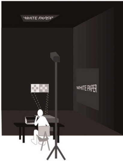
Figure 5. Schematic illustration of the lighting setup used by Zavagno, Daneyko, and Liu [53] in their Gelb-illuminated SLC experiment. The SLC displays were directly illuminated by a theatrical spotlight hidden from the observer’s view. The white paper on the walls and ceiling was positioned for another experiment but not illuminated in the experiment modeled here (adapted from Zavagno, Daneyko, and Liu [53]).
