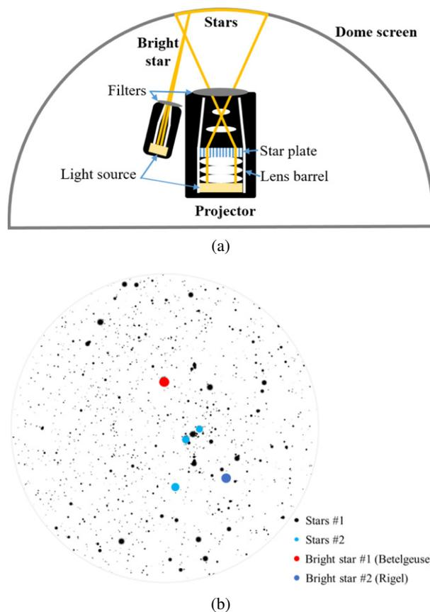
Figure 1. Star reproduction method. (a) System used to project star fields in a planetarium. (b) Representation of the color variation of stars used in our experiment.
