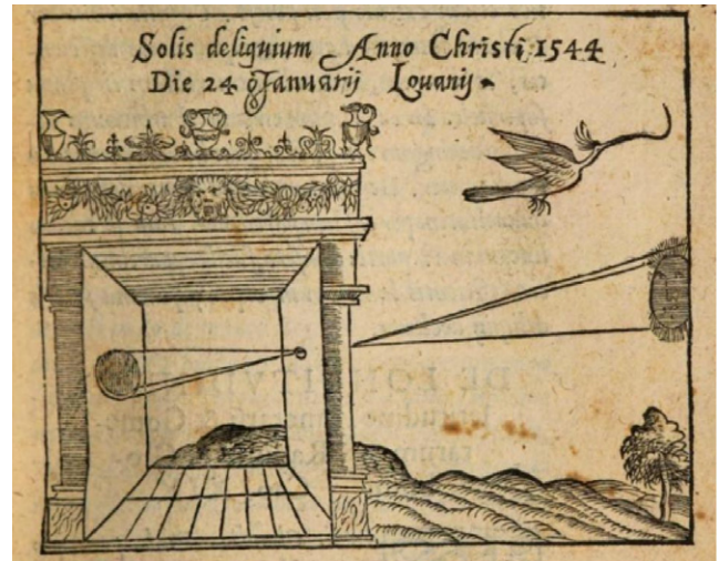
Figure 1. A schematic drawing of the pinhole camera made by Gemma Frisius in 1544 [1].
