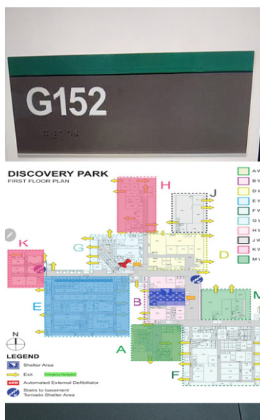
Figure 4. The projected floor plan with wings highlighted when the marker (room number) is scanned.
