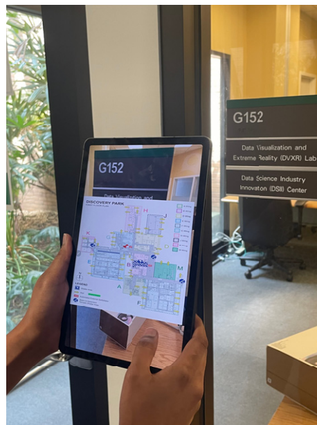
Figure 1. Display of the floor plan in MARA using room numbers as a marker.
