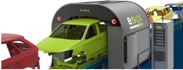
Figure 2. In-line tunnel-type paint defects inspection system esphi [4].
