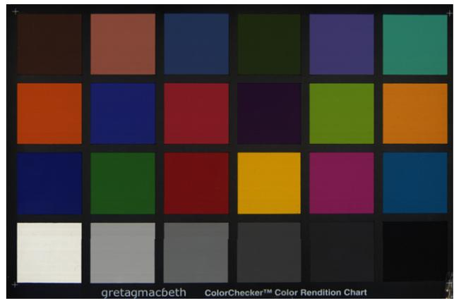
Figure 6. Final photo of hyperspectral camera, all wavelengths (380–780 nm) integrated under illuminant D50.
