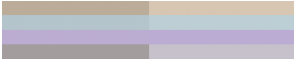
Figure 5. Measured (left) and calculated (right) RGB values of halftoned patches of combinations of primaries under 30° illumination and observation angle. Top to bottom: RG, GB, RB and RGB.
