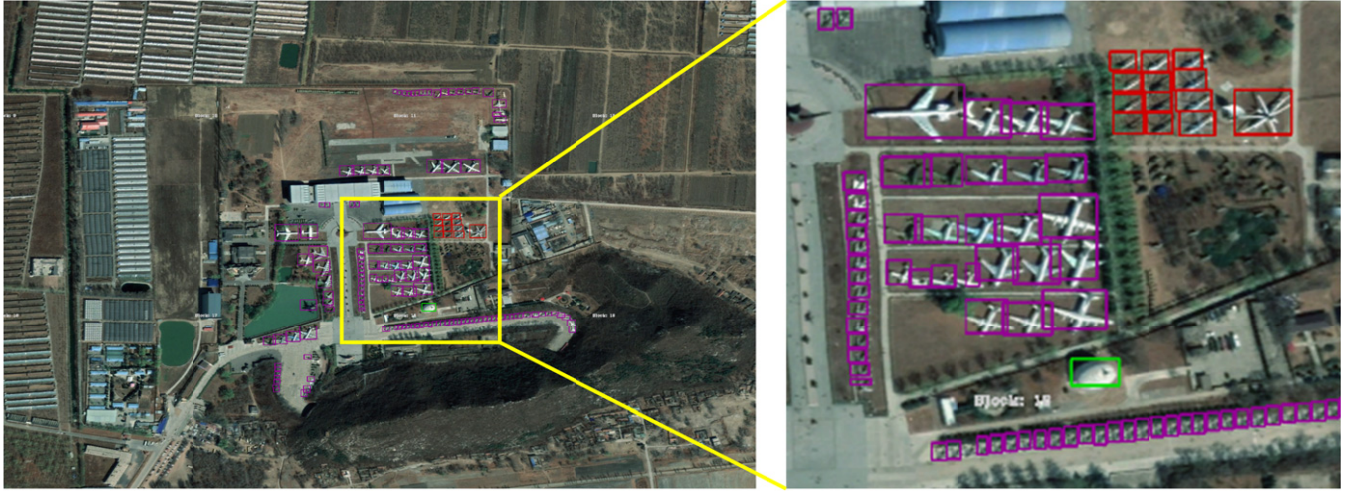
Figure 5. Multiple-target results using YOLOv4-faster.
