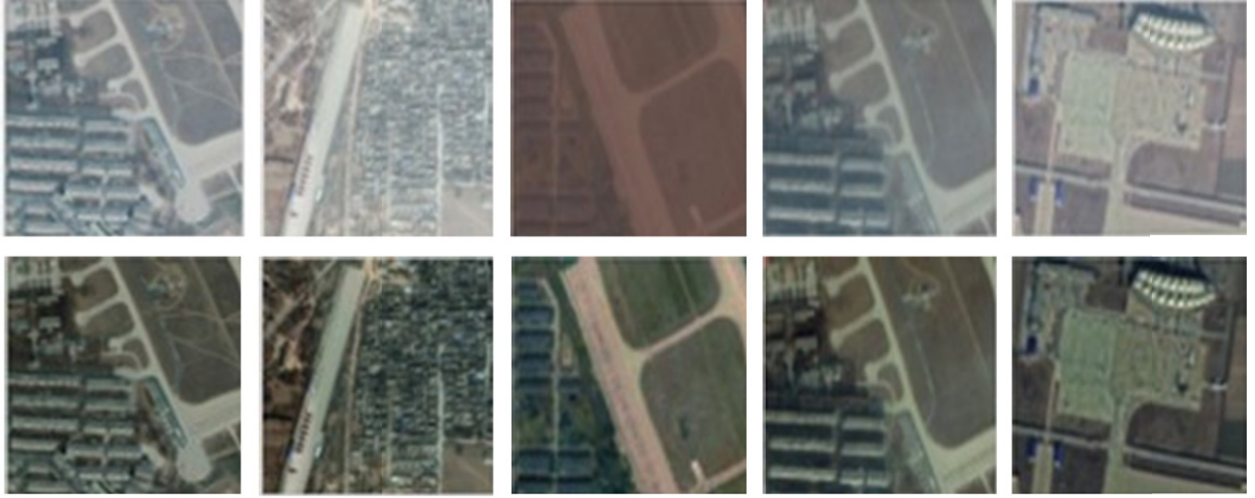
Figure 2. Remote sensing images before and after dehazing.
