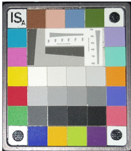
Figure 1. Rez checker target nano matte designed by Image Science associates. The circles are used as reference for automatically determining the regions of interest within the test image. The colored patches are used for measuring color fidelity. The gray patches are used for measuring the noise and the optoelectronic conversion function which is necessary for calculating the modulation transfer function. The gray slanted edges are used for measuring the step response and calculating the modulation transfer function to assess sharpness. Note that images cannot be reproduced with original resolution and color because of degradation associated with various steps for preparation and printing of the manuscript.
