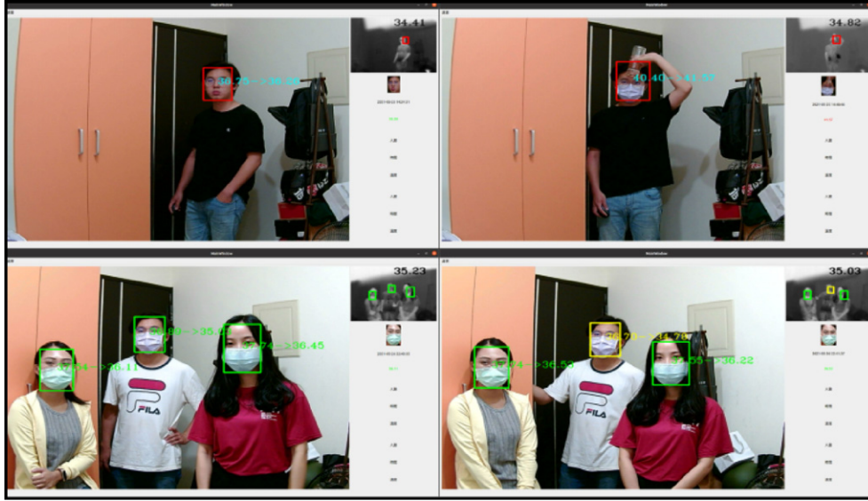
Figure 3. The detection results of the study in a simulated reality scenario. The proposed method is able to detect various face mask-wearing and face temperature with both the surveillance camera and the thermal imaging camera.
