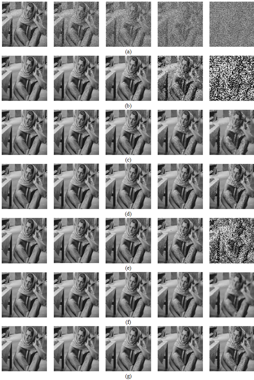
Figure 5. Comparable results: (a) the corrupted Barbara images by salt-and-pepper noise from 10 to 90% with increments by 20 from left to right; (b) corresponding SMF (second row); (c) AMF (third row); (d) IASMF (fourth row); (e) LIO (fifth row); (f) SAM (sixth row); and (g) the proposed approach (seventh row). As the noise density increases, the corresponding results from the compared algorithms give different observations.
