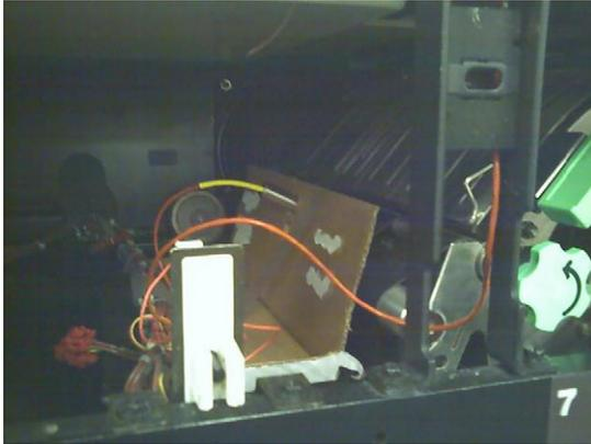
Figure 5a. Picture of the interior of a Xerox Docutech 6180 with sensors placed in the paper path.
