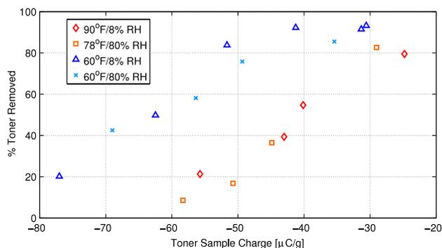
**Figure 7.** Data from toner adhesion testing at 90°F/8% relative humidity; 78°F/80% relative humidity; 60°F/8% relative humidity and 60°F/80% relative humidity. Data is shown as a function of toner charge for each sample, which was manipulated with transfer voltages.
