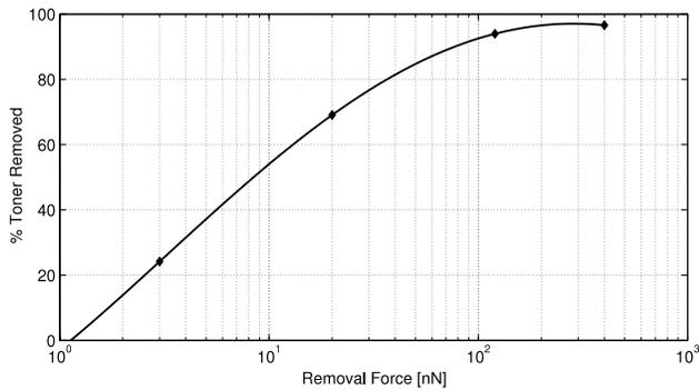
Figure 4. Toner removal as a function of force. The toner is at ambient temperature and humidity (approximately 72°F/50% relative humidity) after being printed onto a polyimide belt sample in a production printer.
