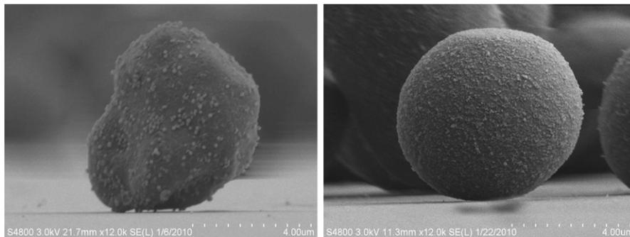
Figure 5. Scanning electron microscope image of weakly held toner particles (i.e. low dispersive adhesion forces).
