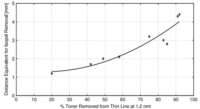
Figure 3. Example of a distance adjustment to correlate the isopel toner removal with thin line toner removal. Multiple samples create a calibration curve for halftone adhesion measurements converting distance values to force at that distance. This is one representative calibration curve used to account for collisions in the isopel samples.
