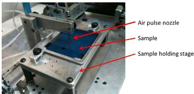
**Figure 2.** Blow-off tool. The air pulse nozzle is a 1 mm diameter stainless steel tube which delivers a 1 s metered pulse of air at a pressure ranging from 10 to 20 psi. The tip of the nozzle is located 4 mm above the sample. The sample holding stage includes a custom-built x-y positioning frame for precise positioning with the nozzle and the imaging microscope.
