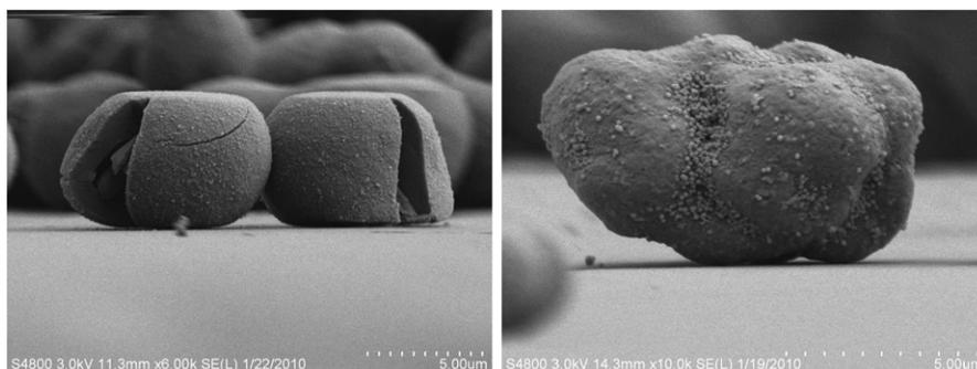
Figure 6. Scanning electron microscope image of strongly held toner particles (i.e. high dispersive adhesion forces).
