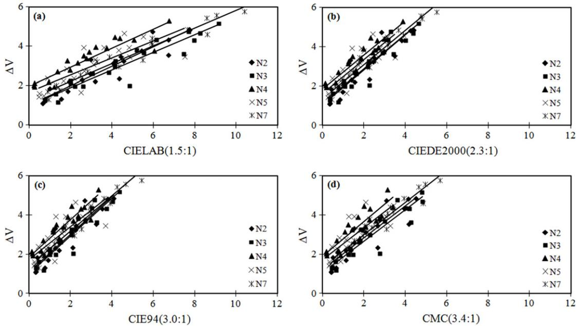
Figure 4. The relationship between visual difference ( $\Delta V$ ) and calculated color difference for color-difference formulas (a) CIELAB(1.5:1), (b) CIEDE2000(2.3:1), (c) CIE94(3.0:1), and (d) CMC(3.4:1) optimized from Experiment I data.
