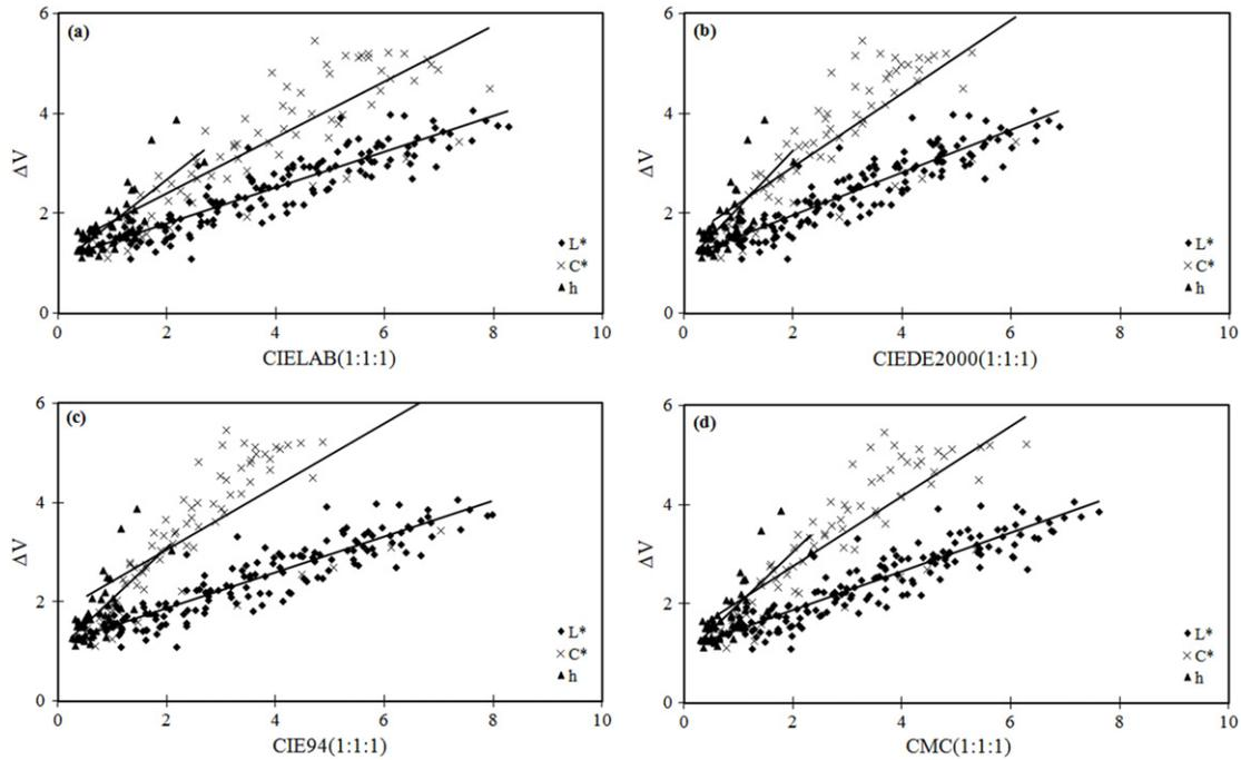
Figure 5. The relationship between visual difference ( $\Delta V$ ) and calculated color difference in lightness, chroma, and hue for (a) CIELAB(1:1:1), (b) CIEDE2000(1:1:1), (c) CIE94(1:1:1), and (d) CMC(1:1:1) from Experiment II data.
