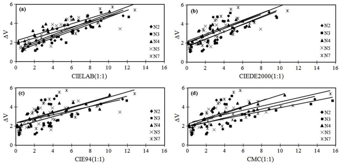
Figure 3. The relationship between visual difference ( $\Delta V$ ) and calculated color difference for (a) CIELAB(1:1), (b) CIEDE2000(1:1), (c) CIE94(1:1), and (d) CMC(1:1) from Experiment I data.
