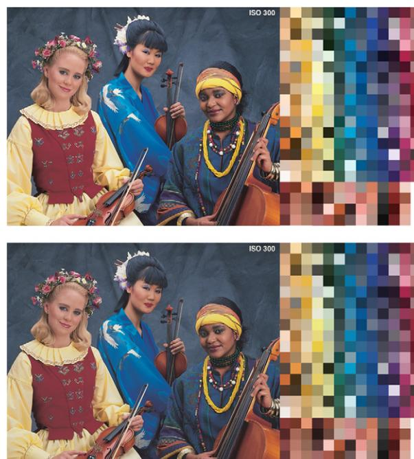
Figure 2. An example of a printed test pair of images (N7: original at the top, modified at the bottom) and their 256 typical color patches; these patches were used to measure the color difference between the two test images.
