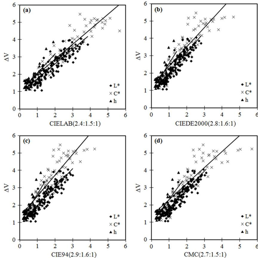
Figure 6. The relationship between visual difference ( $\Delta V$ ) and calculated color difference for color-difference formulas (a) CIELAB(2.4:1.5:1), (b) CIEDE2000(2.8:1.6:1), (c) CIE94(2.9:1.6:1), and (d) CMC(2.7:1.5:1) optimized from Experiment II data.
