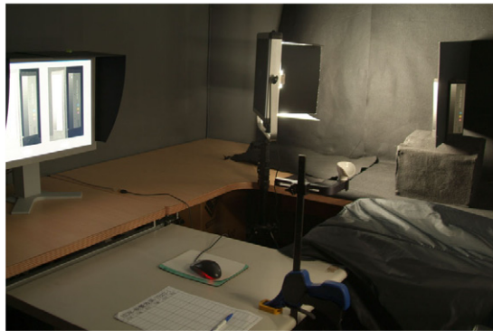
Figure 6. The viewing environment for the paired comparison between the real HDR scene and the reproduced LDR images. (The room light was turned on here for illustration.) The observer can turn 90° to view each side back and forth.
