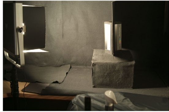
Figure 4. The lighting configuration used in the first experiment. The cool-white fluorescent light set on the left provides much higher illumination than the one on the far right (not seen) to generate HDR conditions.
