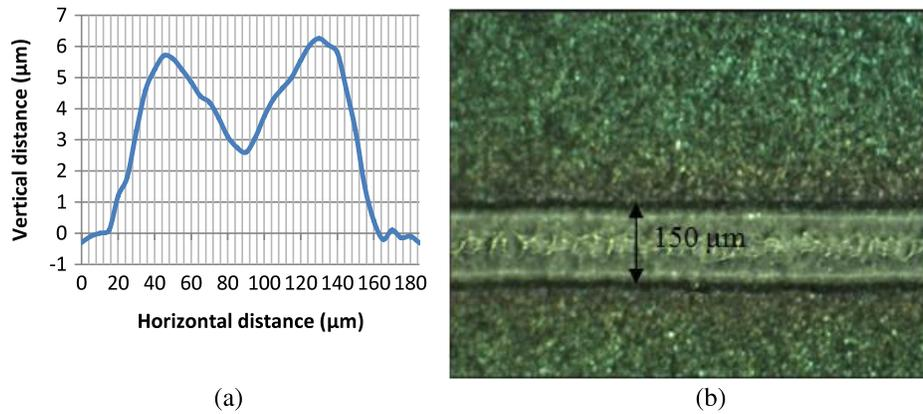
**Figure 6.** (a) Dektak profile and (b) optical image of a printed PAA line. The lines were achieved by printing 8 layers of 1% (w/v) PAA solution on an acidic-textured multicrystalline wafer using a 150  $\mu\text{m}$  nozzle. The AJP settings used were (i) SFR = 20 sccm, (ii) AFR = 30 sccm, and (iii) 5 mm/s process velocity.
