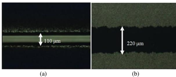
**Figure 7.** (a) Optical microscope image of a printed PAA line with 12.5  $\mu\text{m}$  height after printing and (b) its corresponding isolation line after lift-off. The printed line in (a) was formed by printing 12 layers of 1% (w/v) PAA solution at a process velocity of 3 mm/s. Other printing parameters were (i) SFR = 20 sccm, (ii) AFR = 30 sccm, and (iii) 200  $\mu\text{m}$  nozzle. The aluminum layer thickness is 1.5  $\mu\text{m}$  and lift-off was performed in 30°C solution for 15 min.
