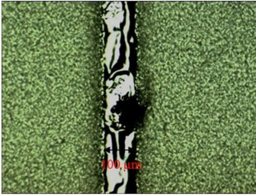
Figure 11. Optical microscope image of a resin line with a height of  $10\ \mu\text{m}$  covered by aluminum after 5 s sonication. On the creation of a crack in the metal, the exposed masking polymer begins to dissolve.
