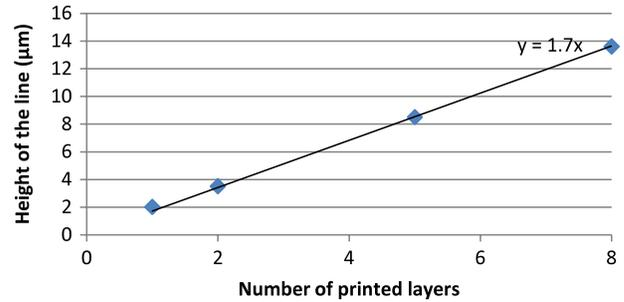
Figure 5. The relationship between the number of printed layers and the resulting height of a printed novolac line when the processing velocity was 5 mm/s on a silicon nitride surface of an alkaline-textured monocrystalline silicon wafer. Other printing parameters were (i) SFR = 30 sccm, (ii) AFR = 1930 sccm, (iii) IE = 1900 sccm, and (iv) 200 μm nozzle.
