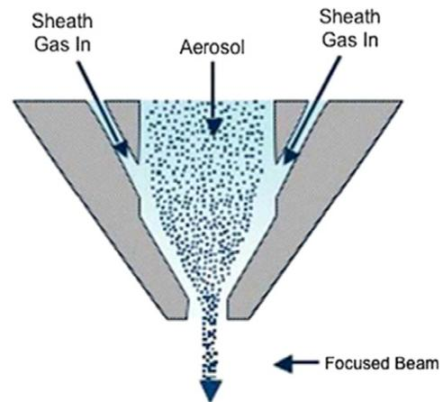
Figure 2. A schematic of atomized material flow and the sheath gas flow in the deposition head of an AJP (reproduced with permission from Optomec Inc.).
