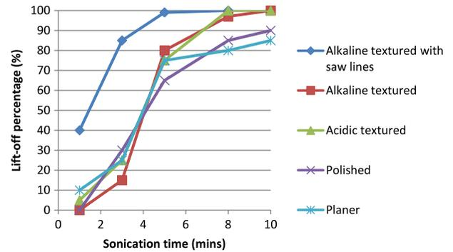
Figure 10. Lift-off percentage versus sonication time for five different silicon nitride coated surfaces with the same masking line height and width. The aluminum layer thickness was 1.2  $\mu\text{m}$  and the lift-off solution temperature was 20°C.
