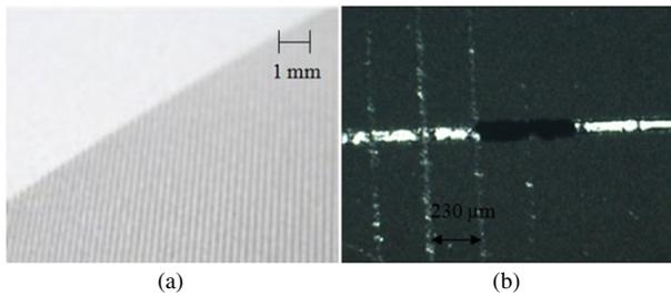
Figure 9. (a) Visible saw lines on monocrystalline wafers and (b) the negative influence of the saw lines on the lift-off process if the masking line is not sufficiently thick and wide.
