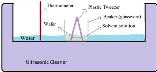
Figure 3. Schematic diagram showing the set up for the sonication process.
