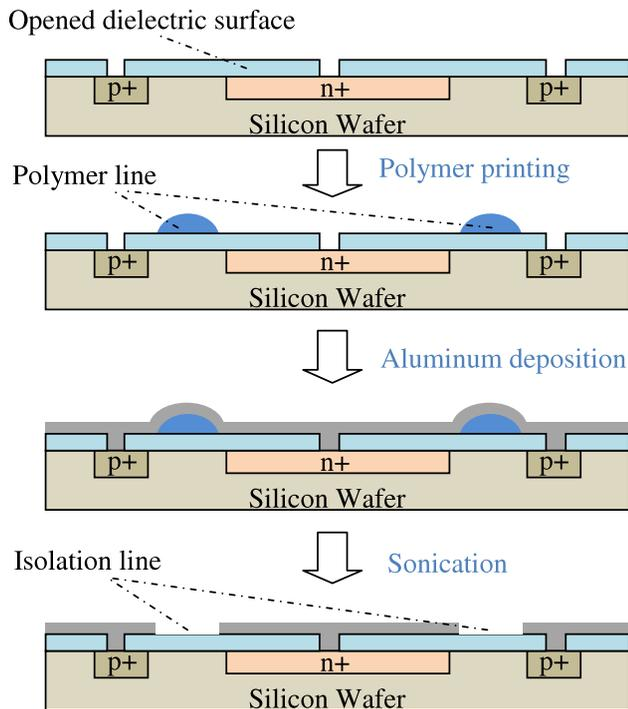
Figure 1. A schematic showing the steps involved in the lift-off process.
