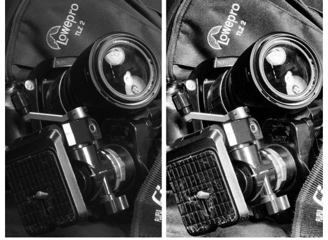
Figure 2. The STRESS algorithm applied to the grayscale image on the left. The image size is 512 \times 779 pixels, and the parameters used were R = 300 , M = 3 , N = 100 .
