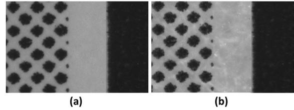
Figure 3. Microscale images with 35% reference coverage, unprinted paper, and 100% ink stripe, (a) reflected image; (b) transmitted image.
