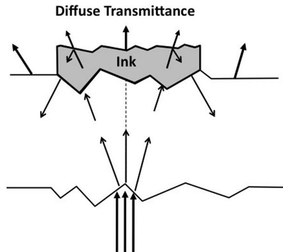
Figure 9. Diffuse transmittance when the light is illuminated perpendicularly.
