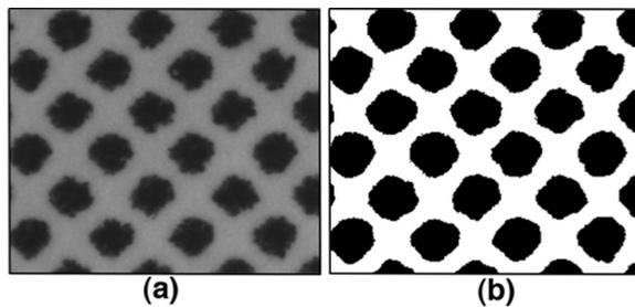
Figure 8. (a) The microscale image of 35% halftone patch printed on coated paper. (b) The effective dot area shape.
