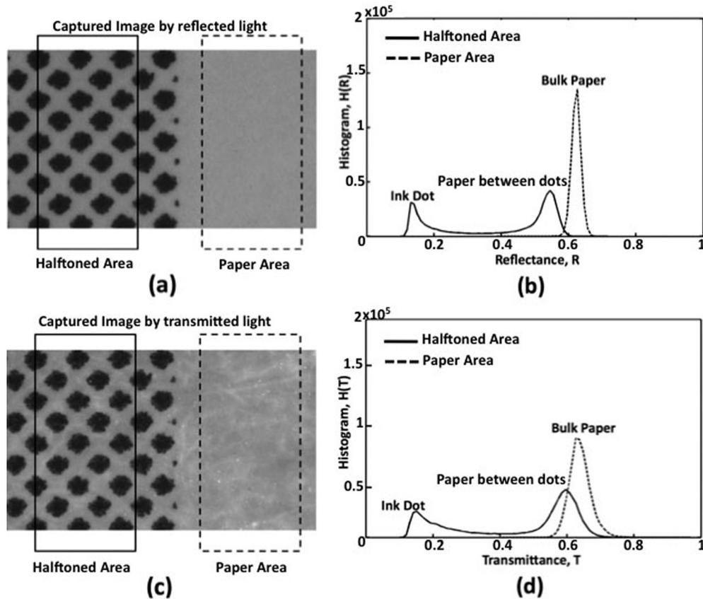
Figure 10. (a) Reflected image for 35% halftone patch. (b) Histograms of halftoned and paper areas in reflected image. (c) Transmitted image for 35% halftone patch. (d) Histograms of halftoned area and paper in transmitted image.
