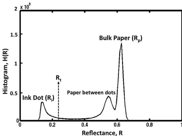
Figure 5. Normalized histogram of the reflected image for 35% halftone patch including bulk paper.
