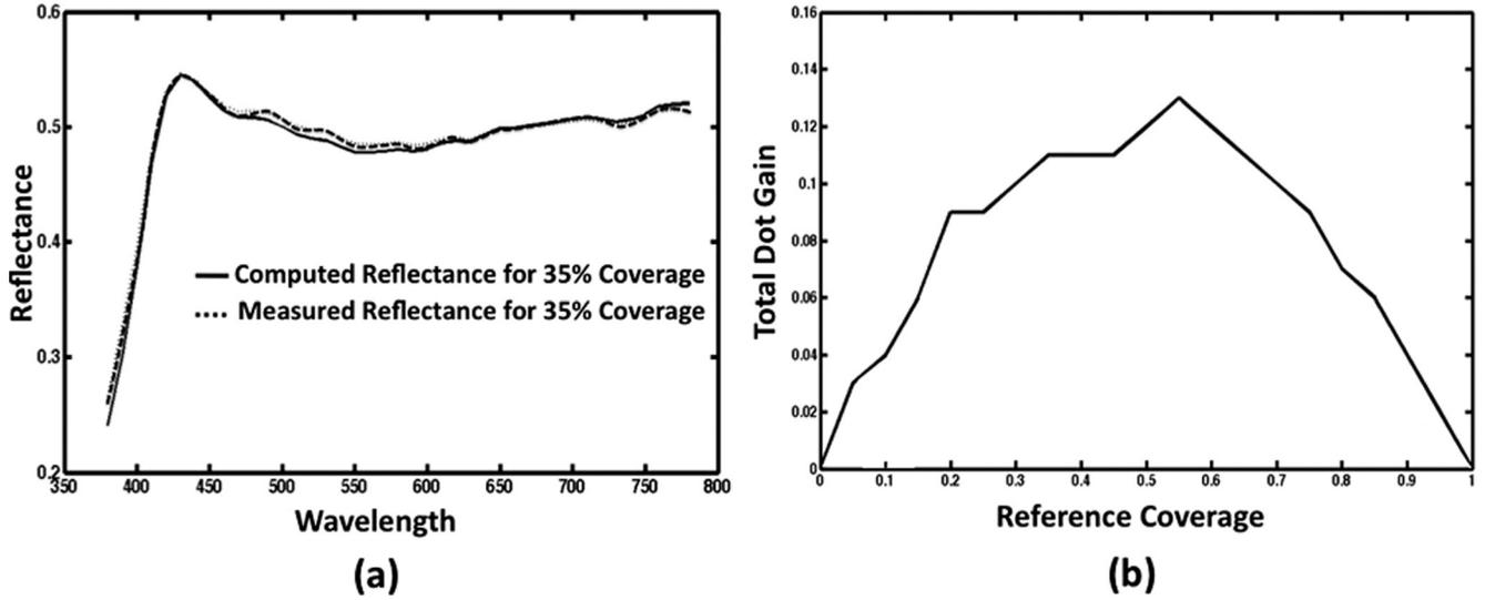
Figure 1. (a) The computed and measured reflectance spectra for 35% halftone patch. (b) The total dot gain computed by the spectroscopic approach.
