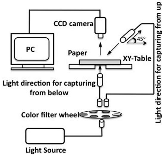
Figure 2. The high resolution camera setup for reflectance and transmittance imaging.
