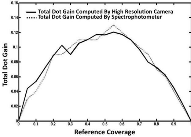
Figure 4. Total dot gain estimated by microscale image and spectroscopic approach.
