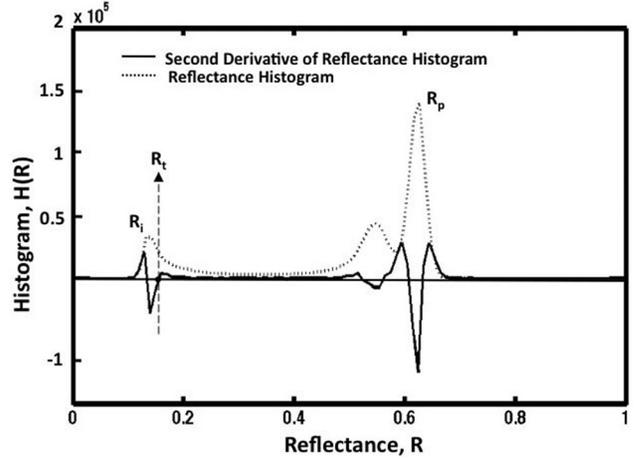
Figure 6. The reflectance histogram (dashed line) and its second derivative (solid line).
