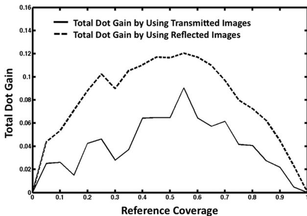
Figure 11. Total dot gain estimated by microscale image approaches: solid line, using transmitted microscale images; dashed line, using reflected microscale images.
