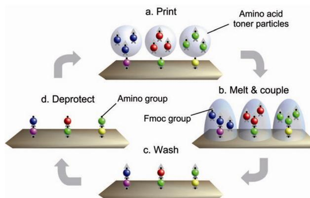
Figure 4. The synthesis cycle includes printing of the amino acid toners (a), coupling of the amino acids by melting (b), washing (c), and deprotecting the coupled amino acids (d).
