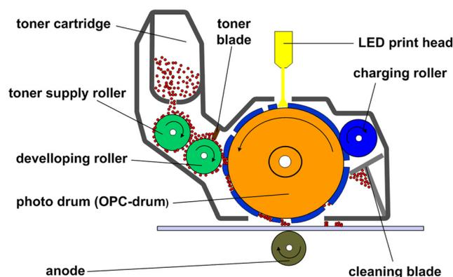
Figure 6. Printing unit: Single-component development system (nonmagnetic) with 1 200 dpi LED-array (Type C2/C4 from Oki Company).
