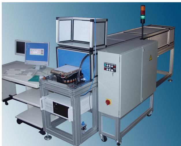
Figure 5. First prototype peptide printer, operated at DKFZ since 2005. Twenty printing units are arranged in a line.
