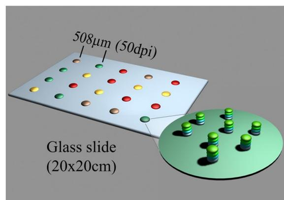
Figure 3. Layer by layer synthesis of a peptide array on a glass slide.
