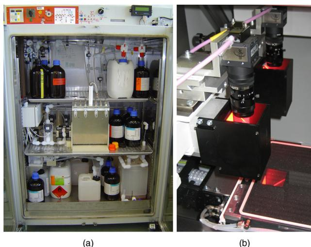
Figure 8. Chemical reactor for processing peptide arrays (left). Vision system for calibration of the printing units, positioning of the glass slides, and reading of bar codes for identification (right).
