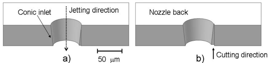
Figure 12. Diagram showing the nozzle geometry and the position and size of nozzle defects (square notches). In (a) a notch of  $4 \times 4 \mu\text{m}^2$  is shown. In (b) a notch size of  $9 \times 12 \mu\text{m}^2$  is shown and it is evident that for this size the defect just starts to affect the rear face of the conical nozzle inlet.
