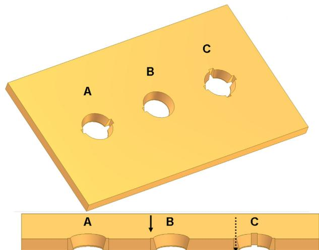
Figure 4. Examples of symmetrical patterns machined on the nozzles of a Xaar XJ 126 printhead by UV laser pulses. In (a), a nozzle with opposed notches across the nozzle axis is shown. (b) A single notch on a side of the nozzle. (c) shows a nozzle where opposed notches have been machined on both the vertical and horizontal axes. Notches were machined perpendicular to the nozzle plate, as indicated by the arrows.
