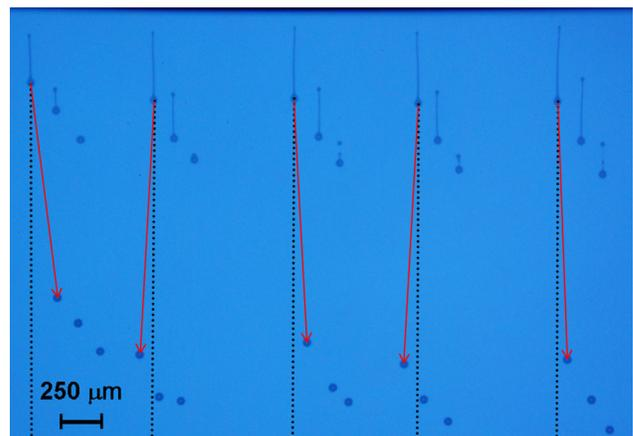
Figure 7. Double-flash shadowgraph images showing the direction of jetting. This image shows 12 jets produced by a Xaar 126 XJ printhead.
