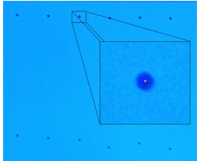
Figure 6. Double-flash shadowgraph image showing a set of six droplets jetted from the Spectra Dimatix SE-128 printhead. Six droplets are observed in the top row and the same six droplets are imaged at the bottom  $700 \mu\text{s}$  later.
