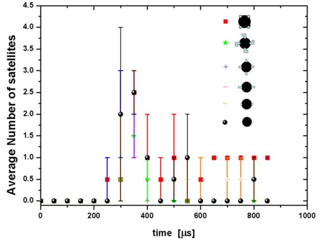
Figure 15. Number of satellites produced by symmetrically modified and unmodified nozzles. For these experiments, droplets were jetted at 3.5 m/s.
