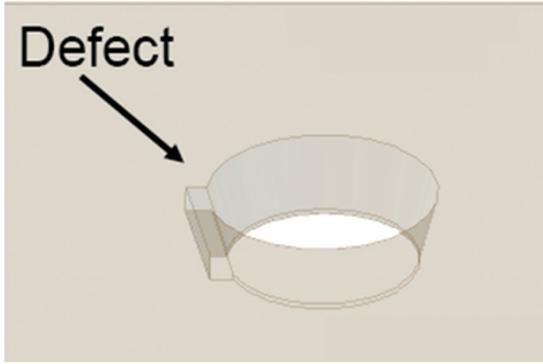
Figure 13. Schematic diagram of a notch parallel to the nozzle surface.
