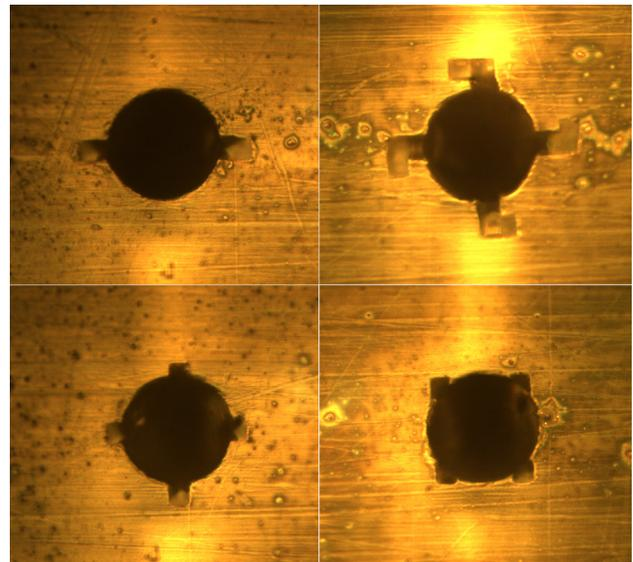
Figure 3. Examples of symmetrical patterns machined on the nozzles of a Xaar XJ 126 printhead by UV laser micromachining (optical images). In these optical images, some residues of the jetting fluid are present in the notches.
