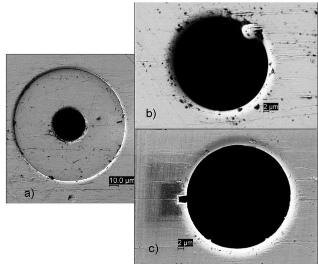
Figure 1. SEM images showing: (a) a Spectra Dimatix nozzle (with a nickel nozzle plate); (b) an example of a typical naturally occurring defect on this printhead; (c) a notch on the side of a nozzle, produced by focused ion beam milling.
