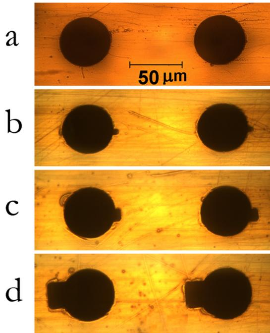
Figure 2. Optical images of nozzles in a Xaar XJ126 DoD nozzle plate: (a) unmodified nozzles; (b) nozzles with notches of  $4 \times 4 \mu\text{m}^2$ ; (c) nozzles with notch sizes of  $12 \times 7 \mu\text{m}^2$ ; and (d) nozzles with notches of  $25 \times 19 \mu\text{m}^2$ .
