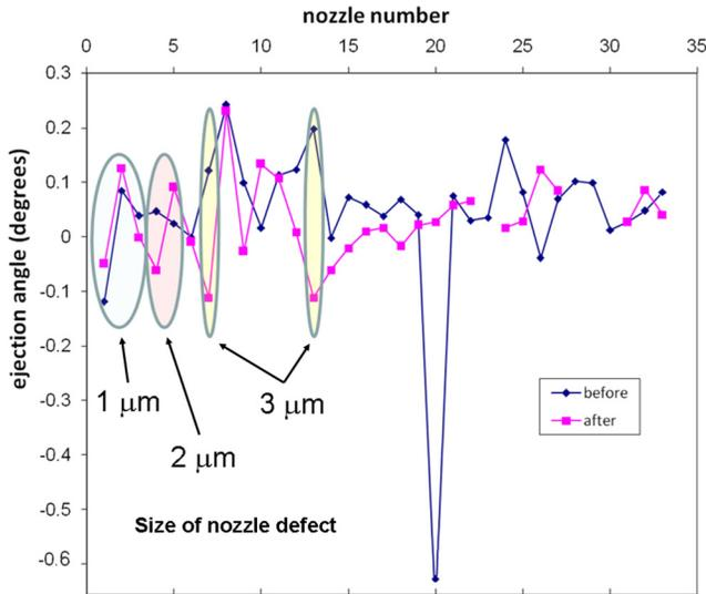
Figure 8. Angles of droplet travel (relative to the nozzle plane normal) before and after nozzle modification by FIB milling. The effect of the changes is noticeable but of similar magnitude to the effect produced by cleaning and refilling of the printhead.
