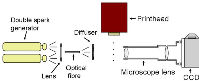
Figure 5. Double-flash shadowgraph system. A Nikon D80 DSLR was used to record the images at a resolution of 10.2 megapixels.
