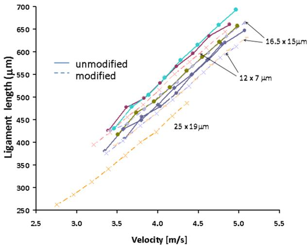
Figure 14. Ligament length plotted against droplet velocity for single side-notches.
