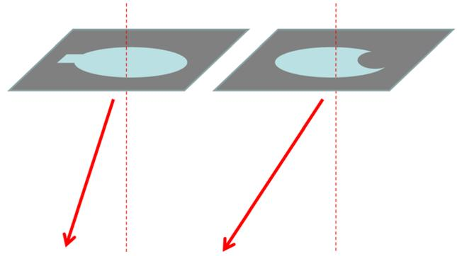
Figure 9. Schematic diagram showing the effects on the directionality of jets caused by the two types of defects on the nozzle plate of a Spectra Dimatix head.
