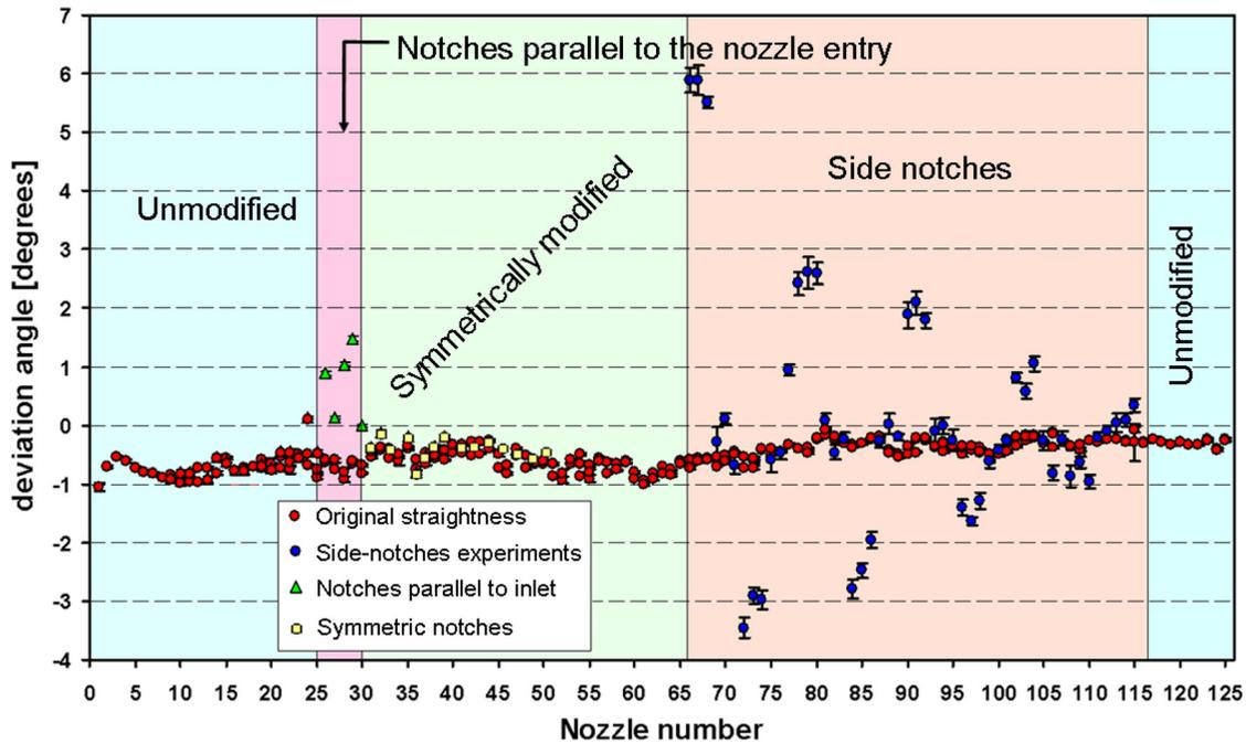
Figure 11. Results of experiments with the nozzles of a commercial printhead modified by laser machining, as described in the text.
