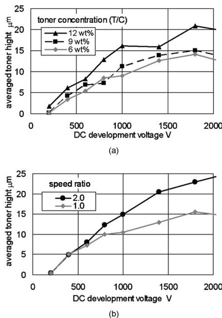
Figure 6. Average toner height of developed toner piles: (a) effect of toner concentration (speed ratio=1.0); (b) effect of speed ratio (toner concentration=6 wt %).
