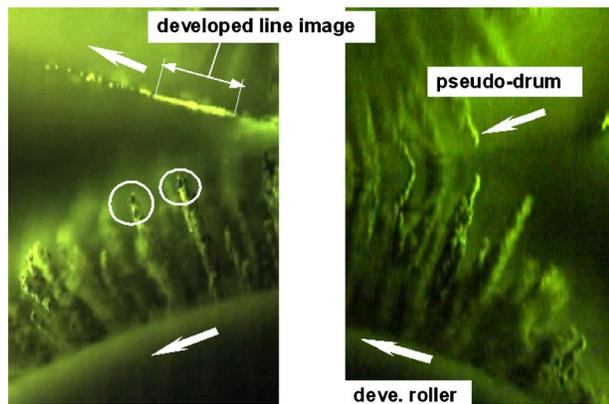
Figure 12. Observed behavior of toner and carrier particles in prenip (inlet) and postnip (outlet) regions of development area ( $T/C$ : 6 wt %; speed ratio: 1.0).
