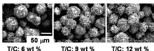
Figure 4. SEM images of mixtures of toner (6  $\mu\text{m}$ ) and carrier (40  $\mu\text{m}$ ) particles.
