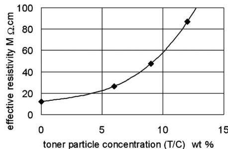
Figure 9. Effective resistivity of mixtures of both carrier and toner particles.
