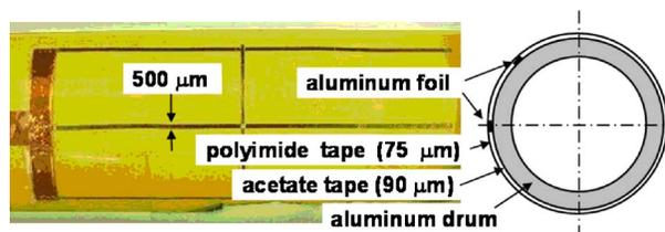
Figure 3. Pseudophotoreceptor drum. Insulated line electrodes made of aluminum foil are embedded on insulated drum.
