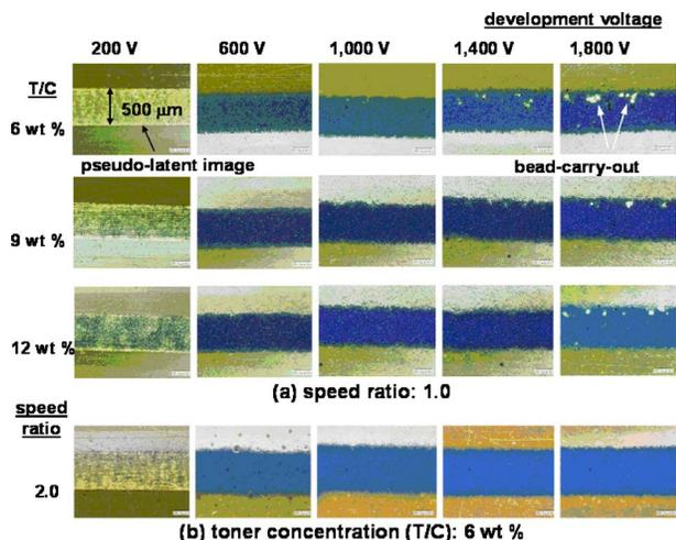
Figure 5. Developed line images on pseudolatent images: (a) effect of toner concentration (speed ratio=1.0); (b) effect of speed ratio (toner concentration=6 wt %).
