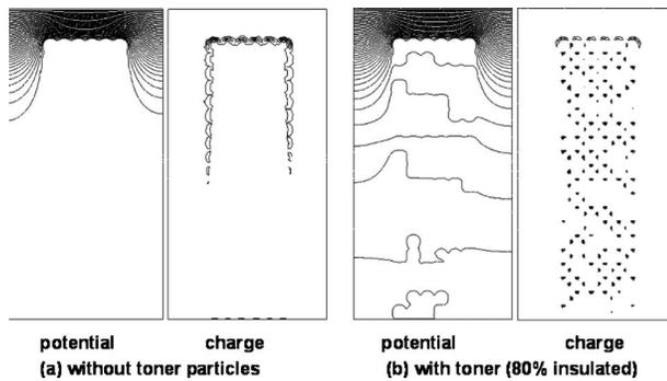
Figure 11. Distributions of steady-state potential and charge density in conductive carrier chain with and without nonconductive toner particles.
