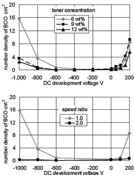
Figure 7. Number density of adhered carrier particles on photoreceptor after development.
