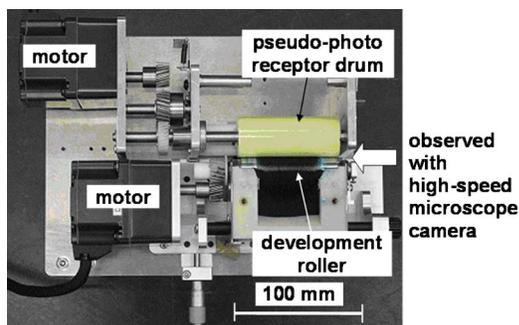
Figure 2. Apparatus used to model a two-component magnetic brush development system.
