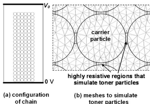
Figure 10. Configuration and dimensions of the calculation domain and the meshes for simulating the presence of toner particles.
