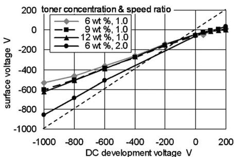
Figure 8. Surface voltage of photoreceptor after development, with respect to dc development voltage.
