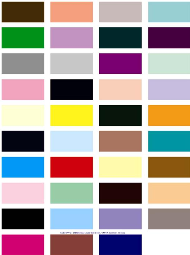
Figure 1. The ISO/IEC 19799 differential gloss test chart (Source: Farnand and Nilosek, "Measurement of Differential Gloss Using a  $\mu$ -Goniophotometer").
