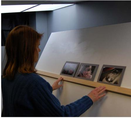
Figure 3. The experimental setup. Half of the bulbs in the outer two sets of lights were illuminated. The remaining lights were turned off.
