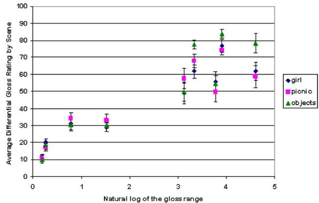
Figure 2. Mean differential gloss rating as a function of the 20° gloss range for each of the nine prints. (Source: Farnand and Nilosek, "Measurement of Differential Gloss Using a  $\mu$ -Goniophotometer").
