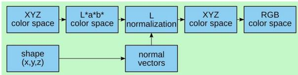
Figure 6. Block diagram of color space calculation process.
