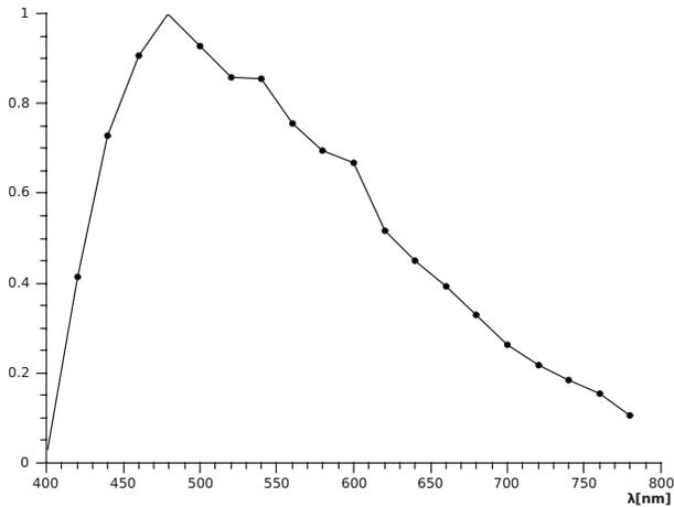
Figure 10. Measured spectral characteristic of xenon light source and optical system attenuation.
