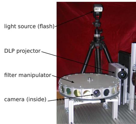
Figure 9. Photograph of the system as built.
