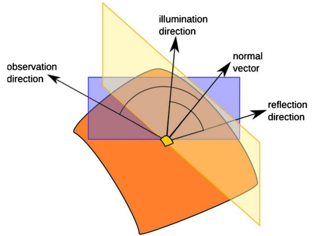
Figure 7. Illustration of illumination and observation directions in relation to surface position.
