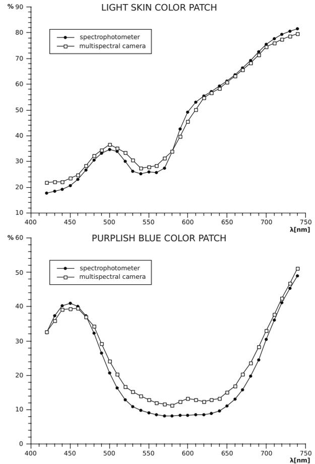
Figure 13. Representative spectral characteristics of GretagMacbeth Color Checker reference plates.
