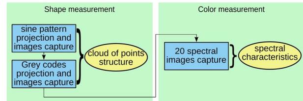
Figure 12. 3D shape and multispectral color measurement sequence.
