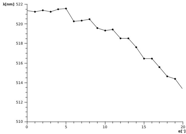
Figure 8. Measured angular characteristic of the interference filter.
