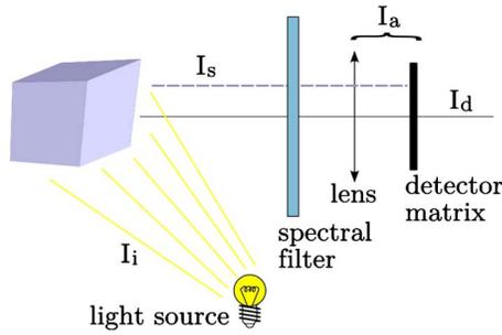
Figure 2. Color measurement system concept.
