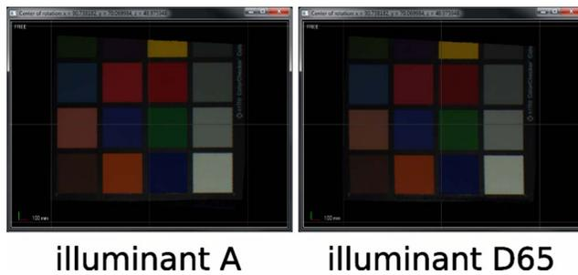
Figure 14. Visualization of the GretagMacbeth Color Checker target measurement result reconstructed under a different standard illuminant.
