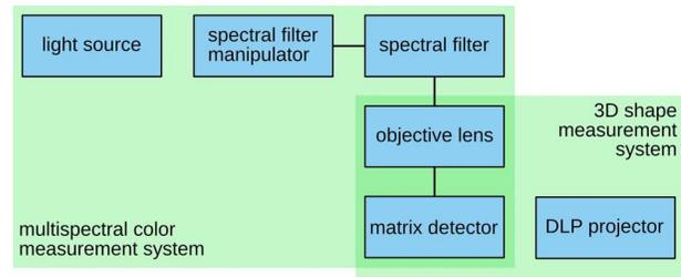
Figure 4. Block diagram of integrated 3D shape and color measurement system.
