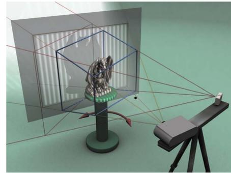
Figure 1. Scheme of 3DMADMAC system with the display of measurement volume indicated as a frustum around the measured object.
