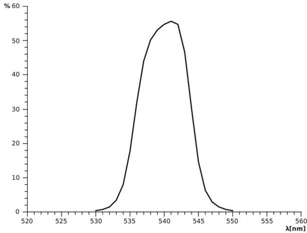
Figure 3. Representative transmission of an interference filter.
