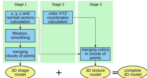
Figure 5. Block diagram of data processing path.
