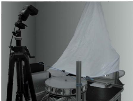
Figure 11. The light tent used for diffuse illumination of the measurement volume.
