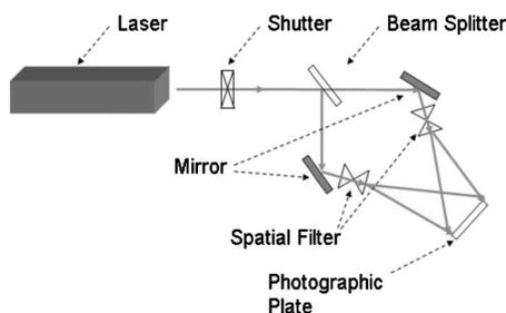
Figure 1. Optical system used to record diffraction gratings.
