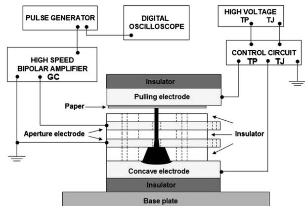
Figure 1. Schematic diagram of the TCB experimental system.
