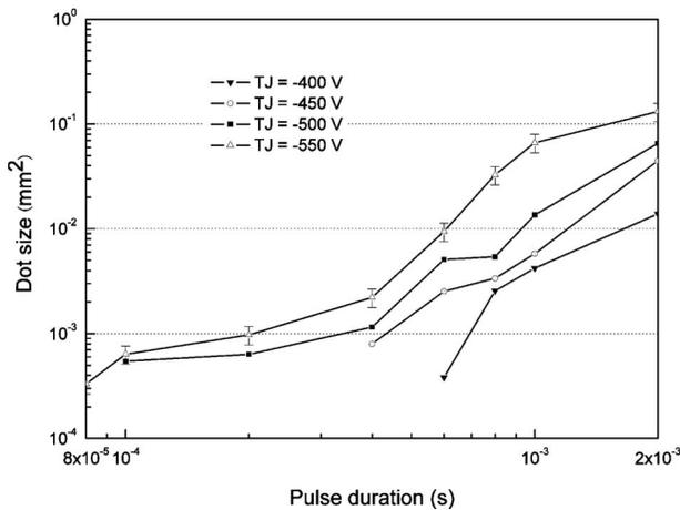
Figure 6. Dependence of dot size on pulse duration plotted on a log scale for four different values of TJ.
