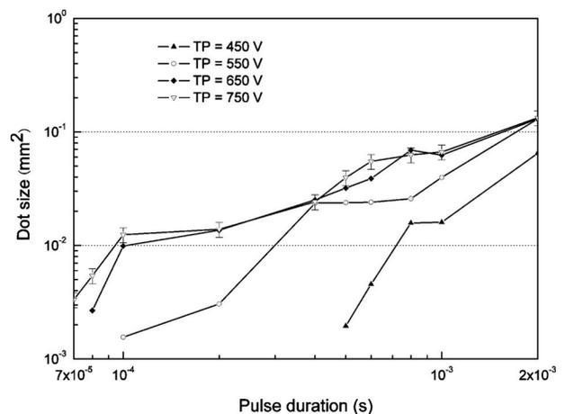
Figure 9. Dependence of dot size on pulse duration plotted on a log scale for four different values of TP.
