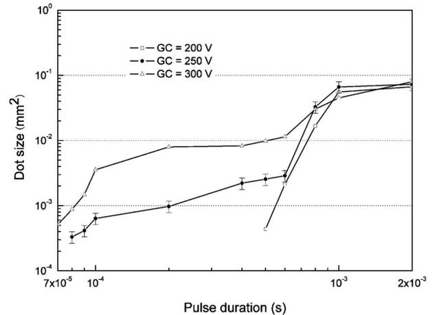
Figure 7. Dependence of dot size on pulse duration plotted on a log scale for three different GC electrode voltages.
