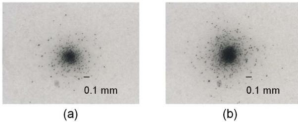
Figure 10. Enlarged images of dots: (a)  $TJ=-500$  V,  $TP=750$  V, and  $t=6 \times 10^{-3}$  s; (b)  $TJ=-500$  V,  $TP=750$  V, and  $t=6 \times 10^{-3}$  s.
