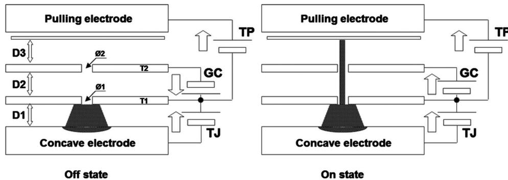
Figure 3. TCB states: (a) off and (b) on states.
