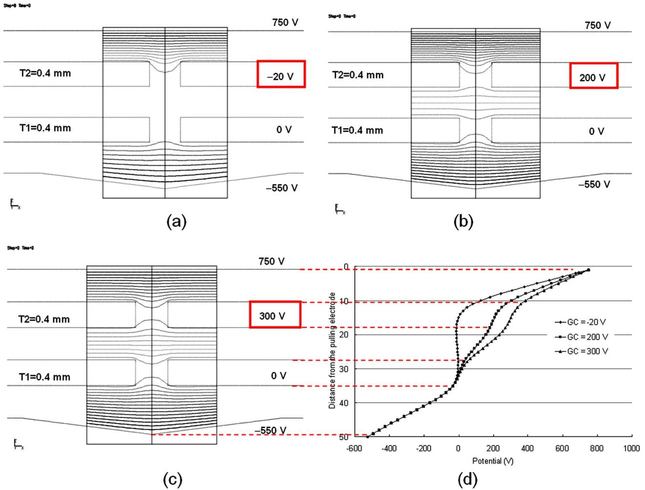
Figure 8. Analysis results for the potential for the (a) off and (b) on states when the GC electrode voltage is 200 V, (c) the on state when the GC electrode voltage is 300 V (equipotential lines are shown), and (d) the potential at the central axis when the GC electrode voltages are -20, 200, and 300 V.
