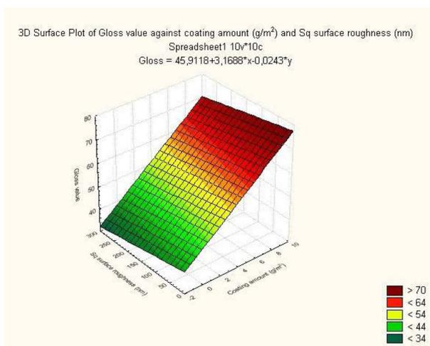
**Figure 2.** Correlation between the gloss and quantity of coating and the gloss and surface roughness of the printed sheets without coating and with three glossy coating amounts.
