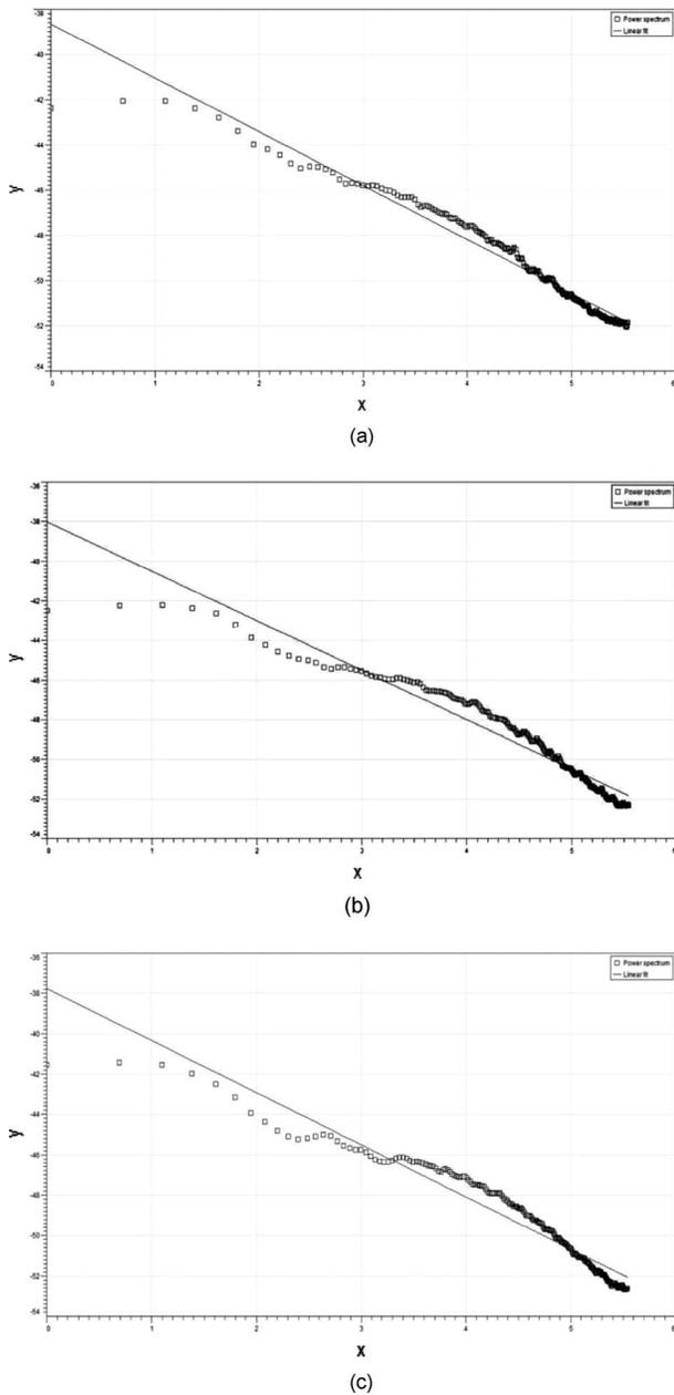
**Figure 6.** PSD graphs of the analyzed surfaces coated with different amounts of UV matte coating by using different screen stencils, with the calculated  $D_f$  values: (a) printed paper coated with the 180 threads/cm stencil,  $D_f=2.24$ ; (b) printed paper with the 150 threads/cm stencil,  $D_f=2.3$ ; and (c) printed paper coated with the 120 threads/cm stencil,  $D_f=2.3$ .
