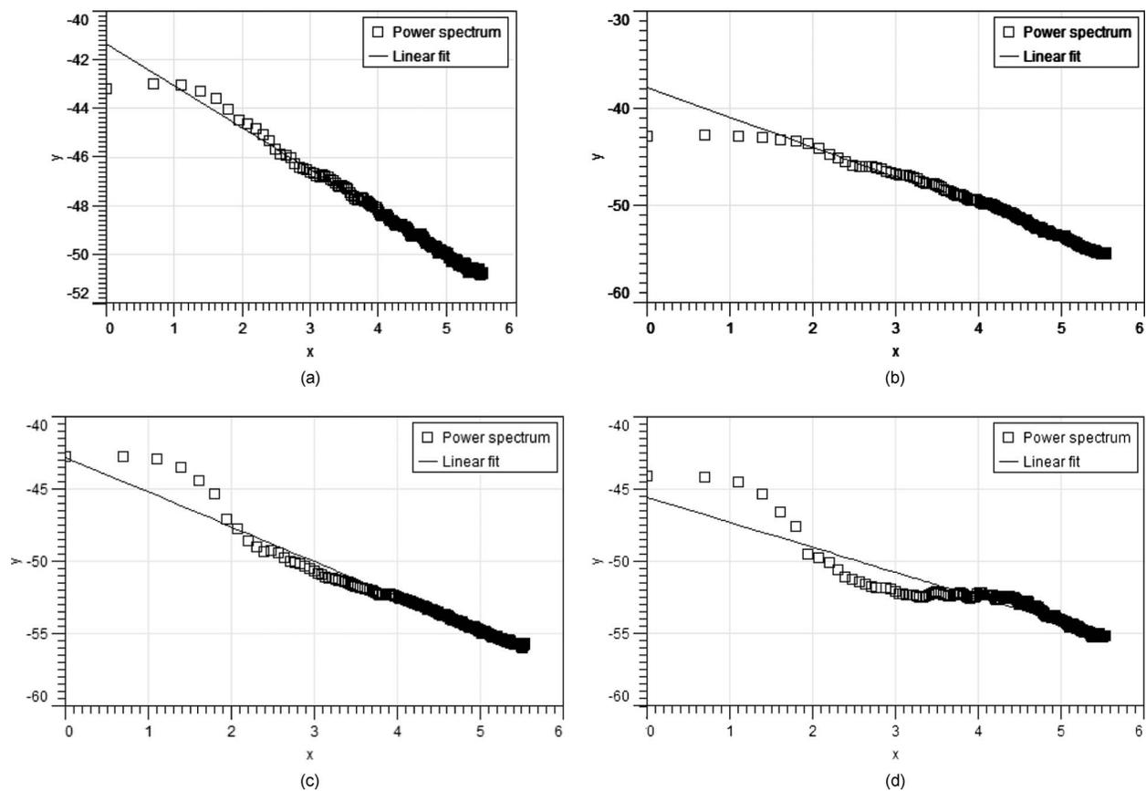
**Figure 5.** PSD graphs of the analyzed surfaces coated with different amounts of UV glossy coating by using different screen stencils, with the calculated  $D_f$  values: (a) plain paper,  $D_f=2.64$ ; (b) ink on paper,  $D_f=1.97$ ; (c) printed paper coated with the 180 threads/cm stencil,  $D_f=2.30$ ; (d) printed paper coated with the 150 threads/cm stencil,  $D_f=2.64$ ; and (e) printed paper coated with the 120 threads/cm stencil,  $D_f=2.75$ .
