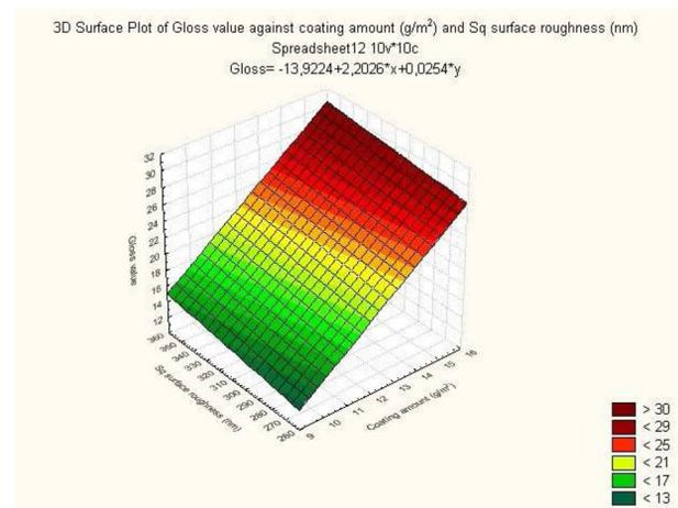
**Figure 3.** Correlation between the gloss and quantity of coating and the gloss and surface roughness of the printed sheets with three matte coating amounts.
