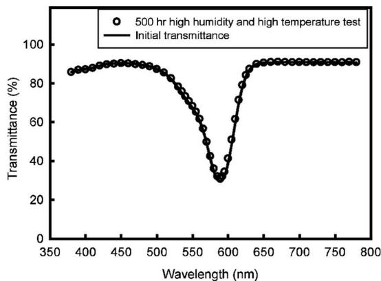
Figure 2. Optical filter durability test.
