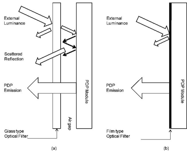
Figure 3. A schematic illustration of light path of PDP TV set: (a) glass-type optical filter; (b) film-type optical filter.
