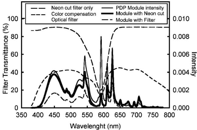
Figure 4. The emission spectrum of a PDP and the transmission spectrum of the optical filter.
