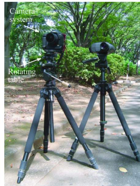
Figure 1. Measuring system for acquiring ambient light properties.
