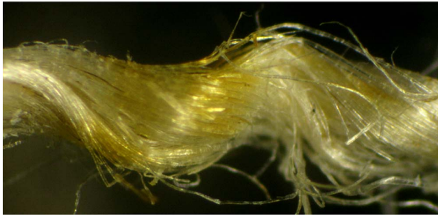
Figure 10. Linen yarn colored with CD: the color intensity varies along the fibers and only the topmost fibers are yellowed.
