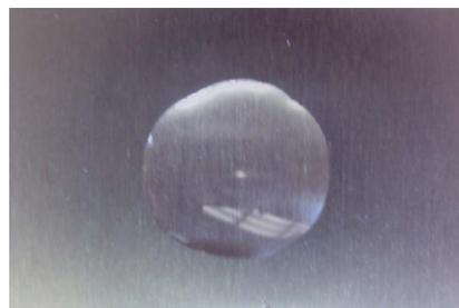
Figure 5. Shape of a water drop on the surface of a dry printing plate.
