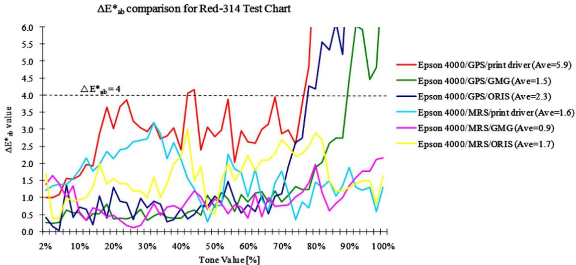
Figure 6.  $\Delta E_{ab}^*$  comparison of original and printed  $L^*a^*b^*$  values for Red-314 chart.
