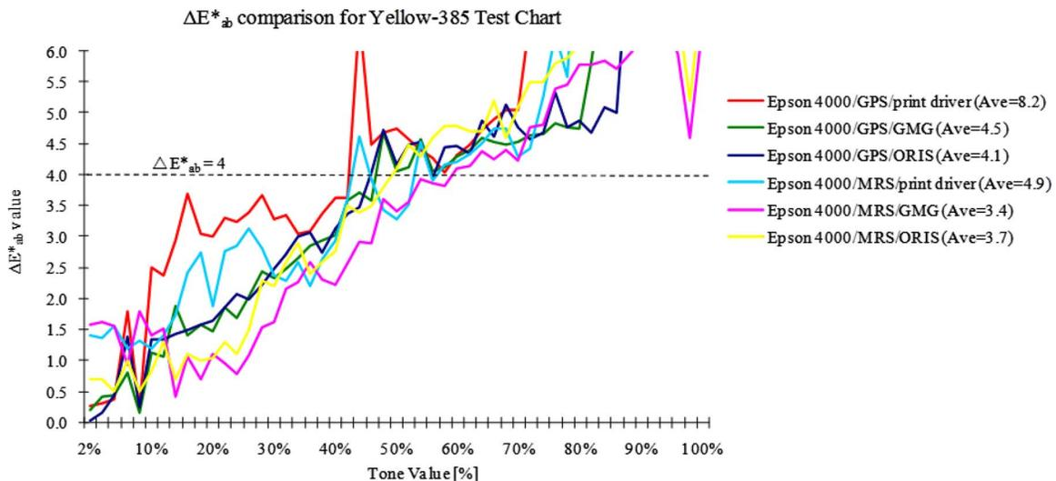
Figure 10.  $\Delta E^*_{ab}$  comparison of original and printed  $L^*a^*b^*$  values for Yellow-385 chart.
