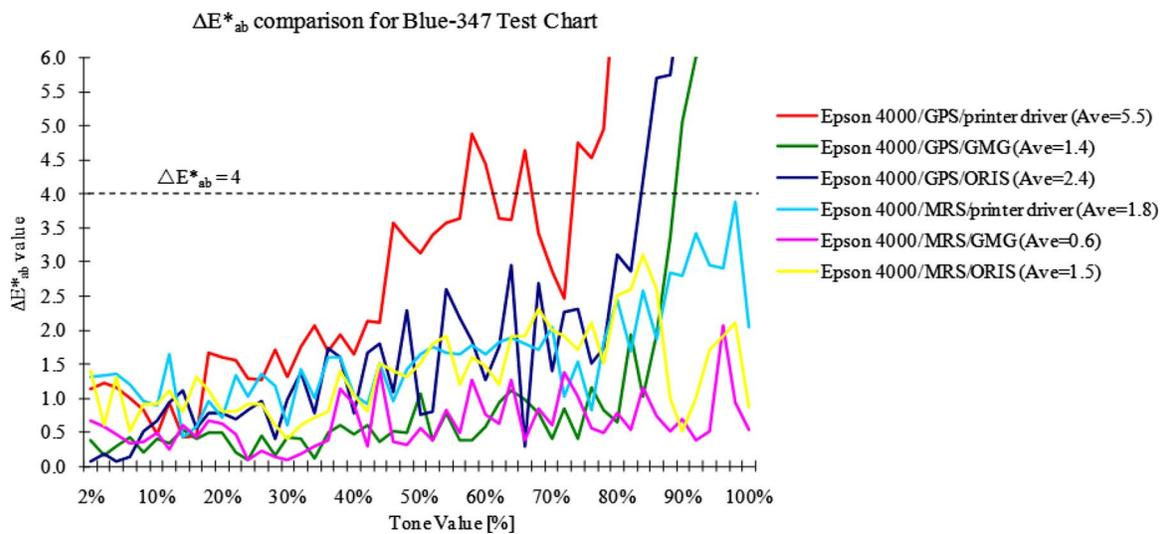
Figure 4.  $\Delta E_{ab}^*$  comparison of original and printed  $L^*a^*b^*$  values for Blue-347 chart.
