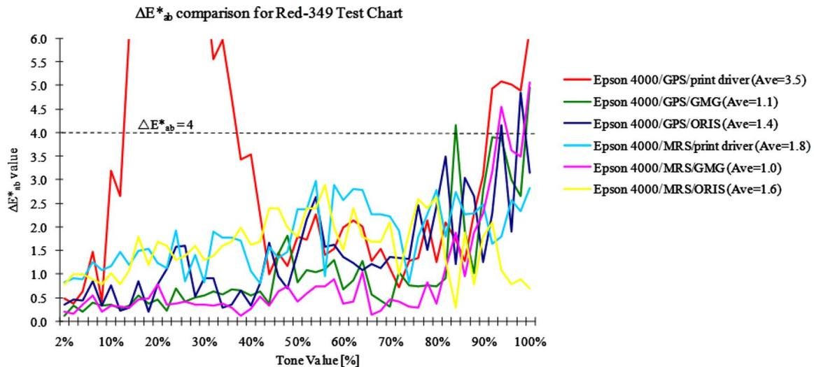
Figure 7.  $\Delta E_{ab}^*$  comparison of original and printed  $L^*a^*b^*$  values for Red-349 chart.
