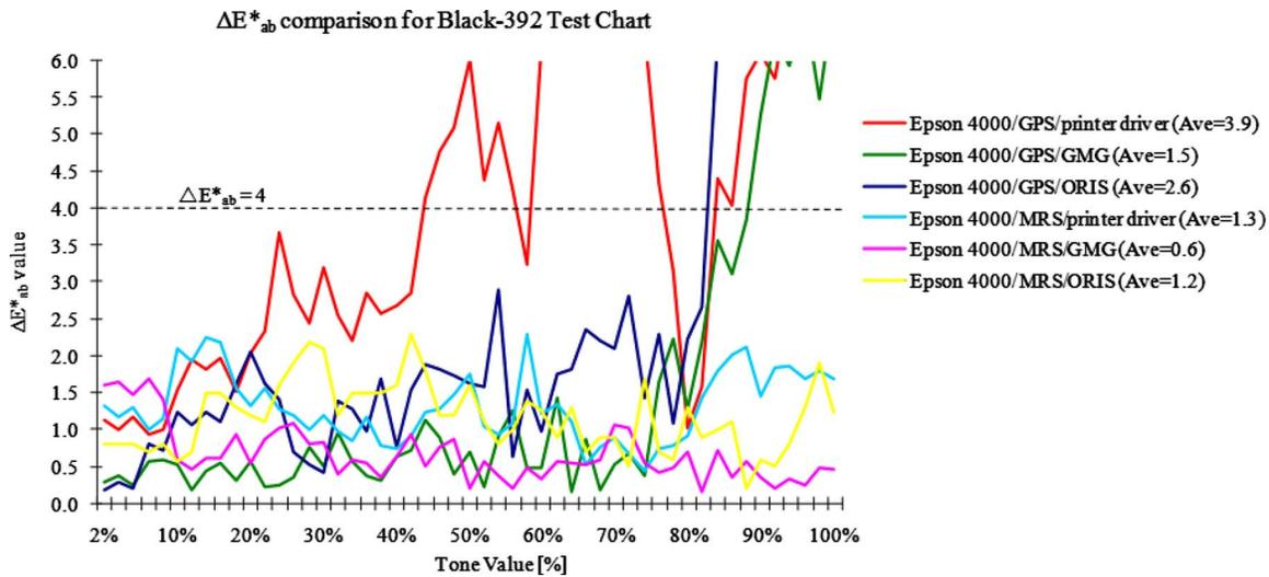
Figure 5.  $\Delta E_{ab}^*$  comparison of original and printed  $L^*a^*b^*$  values for Black-392 chart.
