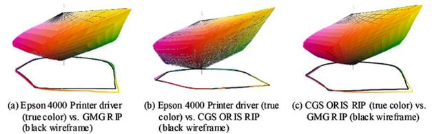
Figure 2. Color gamut comparison on the manufacturer recommended paper for the Epson Stylus Pro 4000 printer. (a) Epson 4000 Printer driver (true color) vs. GMG RIP (black wireframe), (b) Epson 4000 Printer driver (true color) vs. CGS ORIS RIP (black wireframe), and (c) CGS ORIS RIP (true color) vs. GMG RIP (black wireframe).
