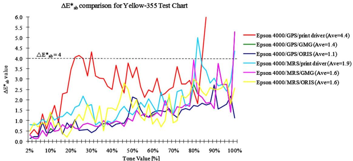
Figure 8.  $\Delta E_{ab}^*$  comparison of original and printed  $L^*a^*b^*$  values for Yellow-355 chart.
