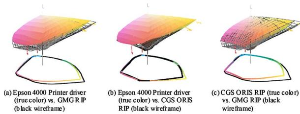
Figure 3. Color gamut comparison on gravure production substrate for the Epson Stylus Pro 4000 printer. The  $L^*a^*b^*$  values of the printed gravure production ink on the production gravure paper are plotted for reference. (a) Epson 4000 Printer driver (true color) vs GMG RIP (black wireframe), (b) Epson 4000 Printer driver (true color) vs CGS ORIS RIP (black wireframe), and (c) CGS ORIS RIP (true color) vs GMG RIP (black wireframe).
