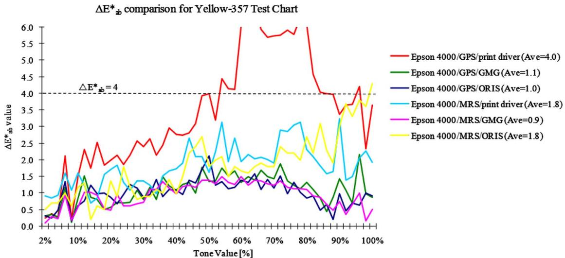
Figure 9.  $\Delta E^*_{ab}$  comparison of original and printed  $L^*a^*b^*$  values for Yellow-357 chart.
