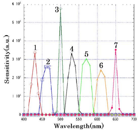
Figure 1. Spectral sensitivities of the sensors of the camera.
