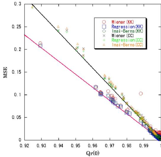
Figure 4. The MSEs of the recovered spectral reflectances by the Wiener, regression, and Imai-Berns method for the GretagMacbeth ColorChecker (CC) and the Kodak Q60R1 (KK) are plotted as a function of  $Q_r(0)$ , which is the value of  $Q_r(\sigma^2)$  when the estimated noise variance is zero. This is the case without consideration for the noise.
