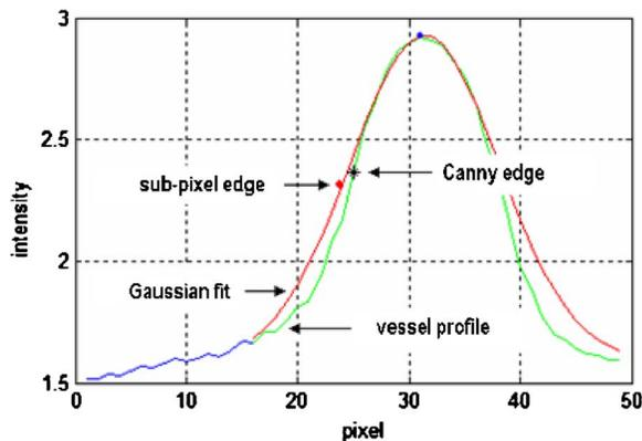
Figure 5. Sub-pixel edge position comparing with Canny edge position with respect to their corresponding vessel cross-sectional profile.
