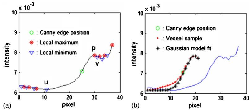
Figure 4. Vessel sample profile determination and Gaussian fit of the profile.
