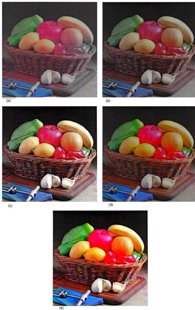
Figure 15. Color images recovered from printed and scanned gray images: (a) color image recovered using conventional method, (b) color image recovered using proposed method without compensation algorithm, (c) color image recovered using proposed method with compensation algorithm when applying characteristic curve, (d) color image recovered using proposed method with compensation algorithm when scaling Cb and Cr components, and (e) color image recovered using proposed method with both compensation algorithm.
