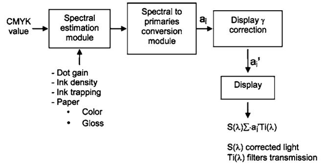
Figure 2. A schematic representation of the spectral display for soft proofing.
