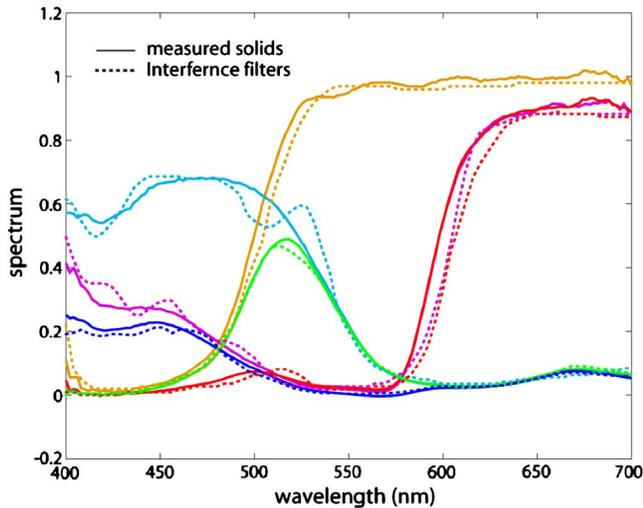
Figure 3. Required vs manufactured filter spectra.
