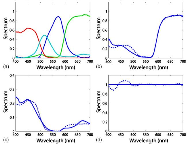
Figure 6. (a) Spectra of the four primaries and (b)–(d) reconstruction of magenta, blue, and white with these four primaries. The other spectra (C, Y, R, and G) are perfectly reconstructed since the primaries spectra are linear combinations of them.
