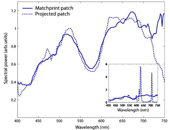
Figure 4. A comparison between the spectrum measured from a Matchprint patch (CMYK=50,41,41,0) and that measured from the spectral display screen. The inset shows the same comparison for a CRT screen under the condition of  $\Delta E=0$  between screen and print (note that the scale of the inset is 5 times larger than the scale of the main figure).
