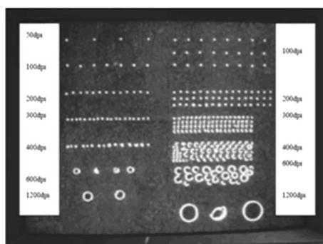
Figure 4. Morphology of the sintered silver nanopaste dot formed by ink jet printing on the P3HT substrate with different drop densities.
