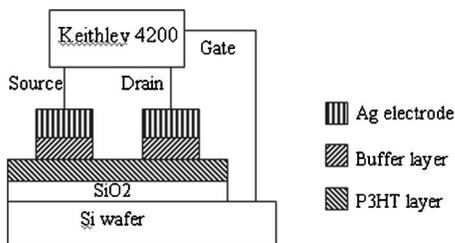
Figure 1. The structure of the polymer thin film transistor device (PTFT) with a silver top electrode.
