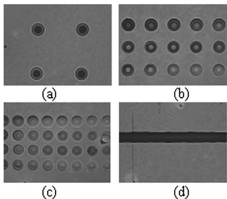
Figure 5. Morphology of the sintered silver nanopaste dot formed by ink jet printing on the V<sub>2</sub>O<sub>5</sub>/P3HT substrate with different drop densities: (a) 100 dpi, (b) 200 dpi, (c) 300 dpi, and (d) 400 dpi.
