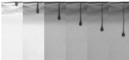
Figure 2. Observation of the break-off behavior of the printed drop beneath an arbitrary nozzle.
