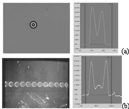
Figure 3. Profiles of the sintered silver nanopaste dot formed by ink jet printing on the different substrates: (a) P3HT and (b) V<sub>2</sub>O<sub>5</sub>.
