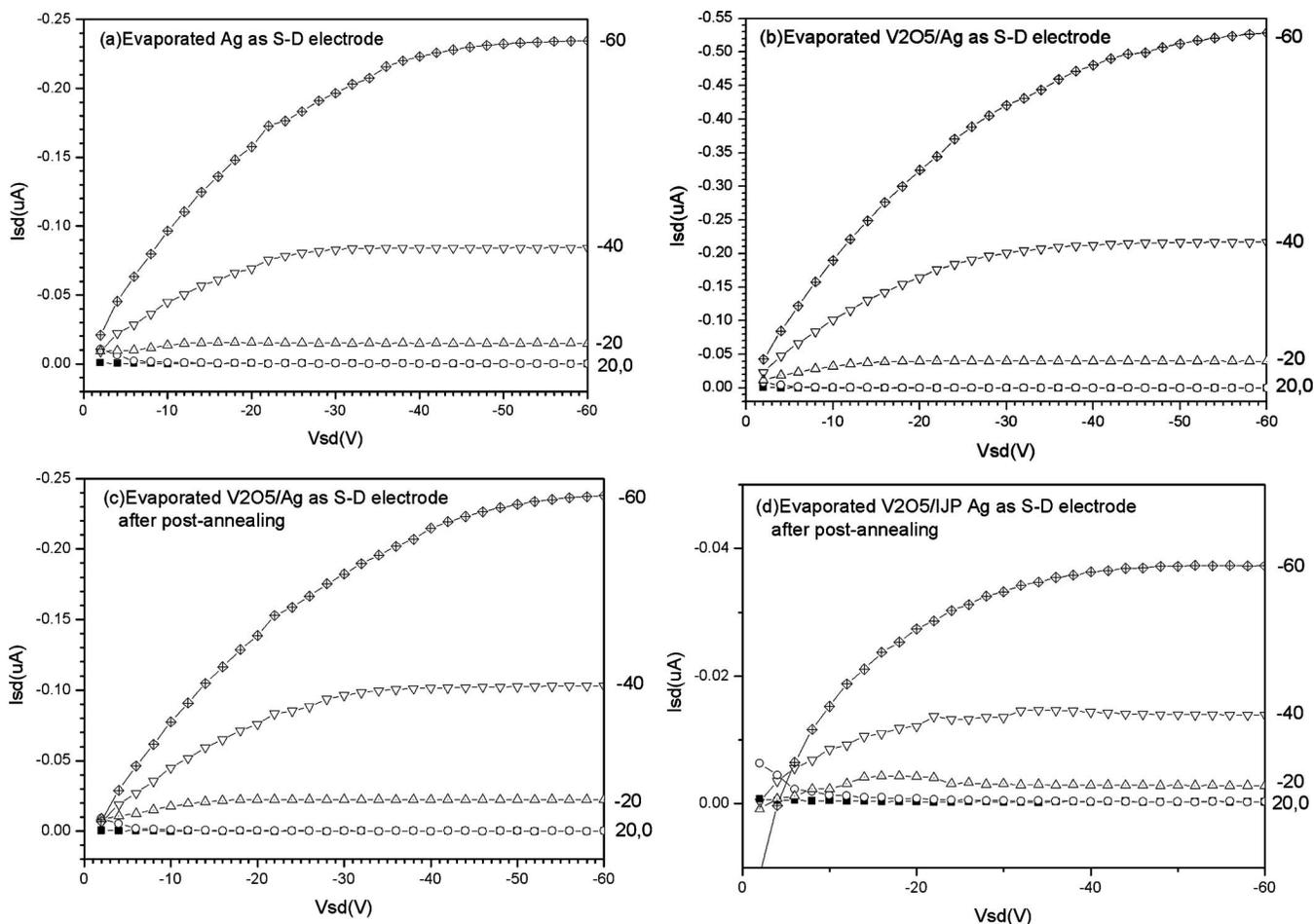
Figure 6.  $I_d$ - $V_{ds}$  characteristics of the PTFT, wherein the source-drain electrodes are: (a) evaporated Ag, (b) evaporated  $V_2O_5$ /Ag, (c) evaporated  $V_2O_5$ /Ag with postannealing, and (d) evaporated  $V_2O_5$ /IJP Ag with postannealing.
