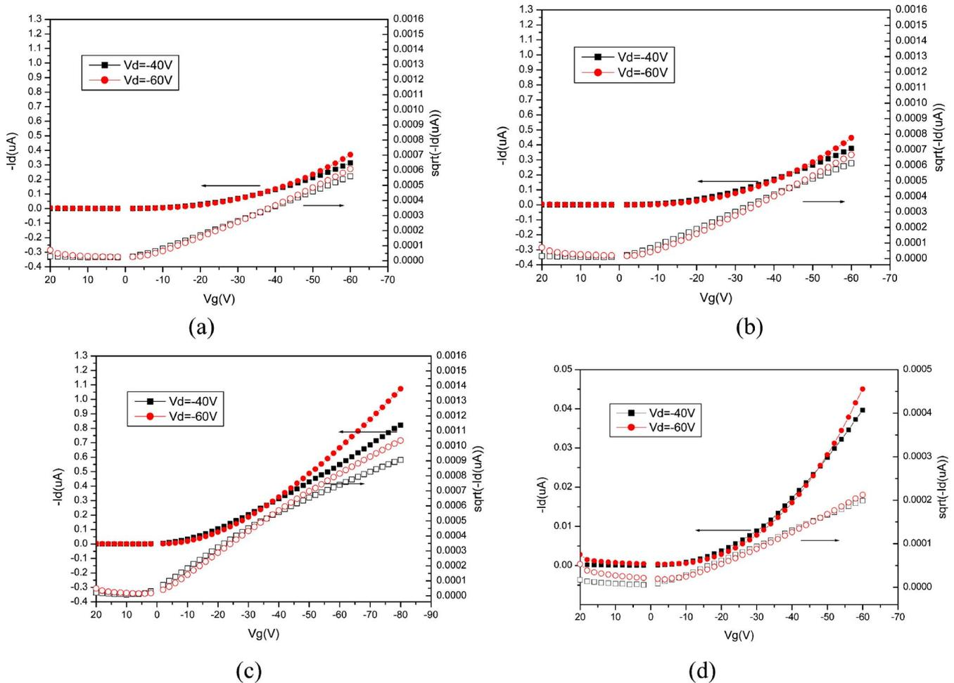
Figure 7.  $I_d$ - $V_{gs}$  characteristics of the PTFT, wherein the source-drain electrodes are: (a) evaporated Ag, (b) evaporated  $V_2O_5$ /Ag, (c) evaporated  $V_2O_5$ /Ag with postannealing, and (d) evaporated  $V_2O_5$ /IJP Ag with postannealing.
