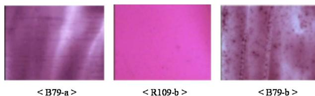
Figure 1. Good dispersion of B79-a and R109-b in comparison to B79-b under an electronic microscope (Scope: 10×0.25).
