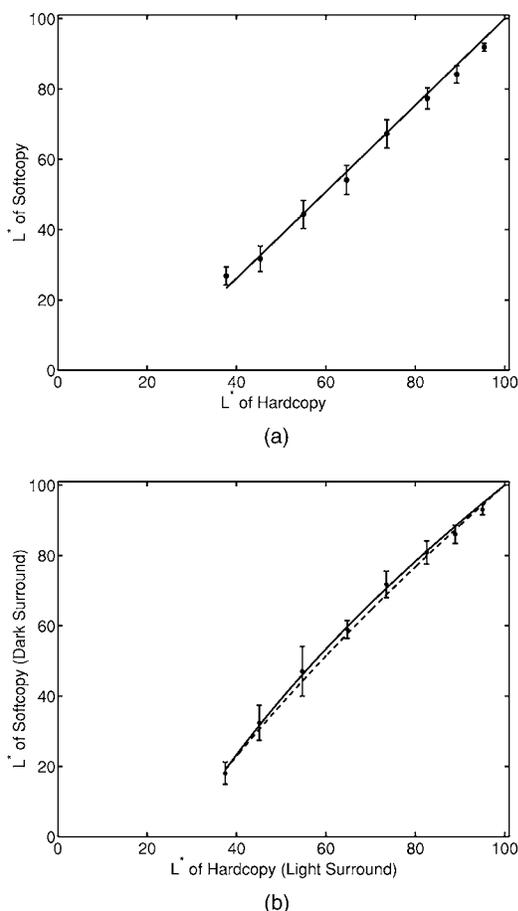
Figure 3. The results of (a) experiment 1, and (b) experiment 2. The solid line is the curve for the experimental data and the dashed line is from previous literature. (Ref. 19). The error bars represent 95% confidence intervals.
