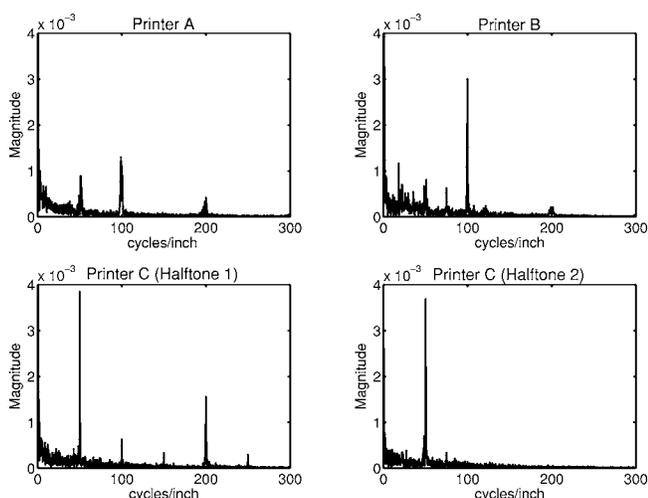
Figure 5. Spectral content of the 1D projection of patches printed with four different printer/halftone combinations.
