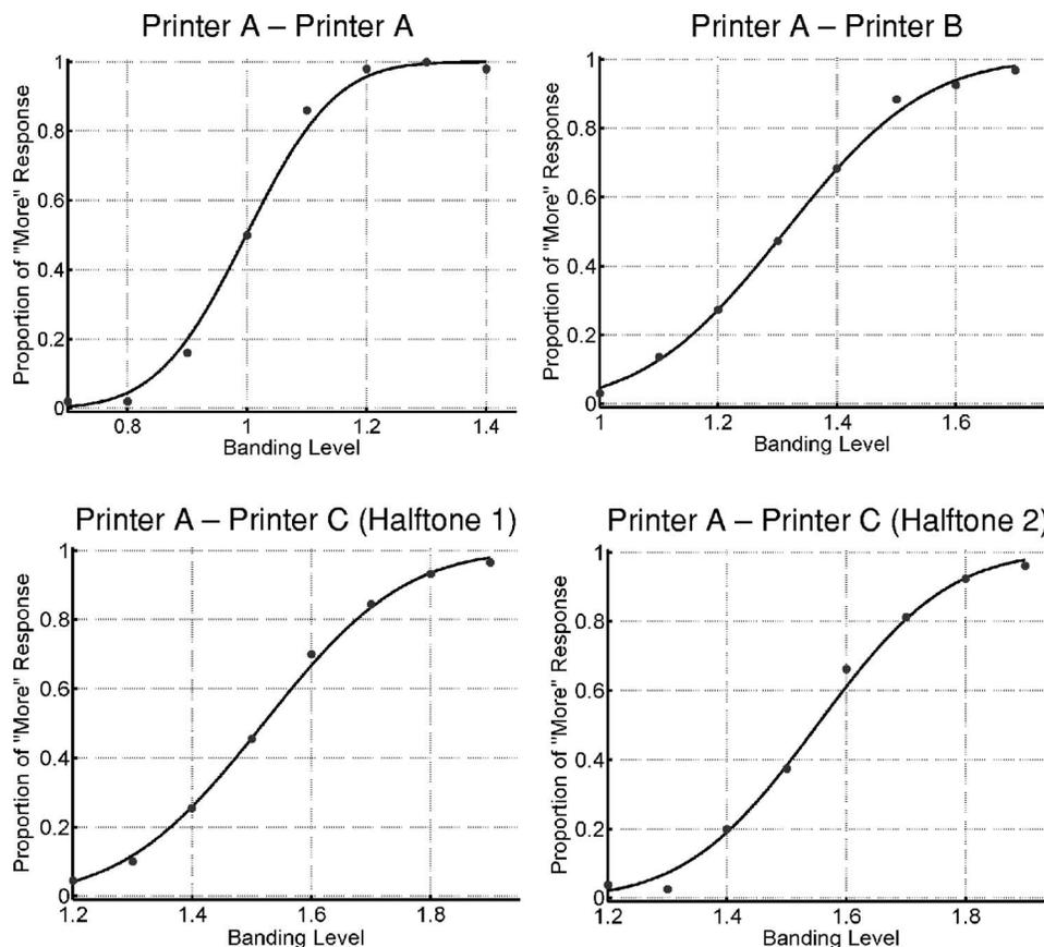
Figure 12. Psychometric functions for the pooled data of the cross platform experiments. The abscissa is the level of banding for Printer A.
