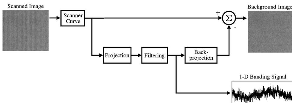
Figure 4. Block diagram for extraction of banding and the background image from the scanned patches.
