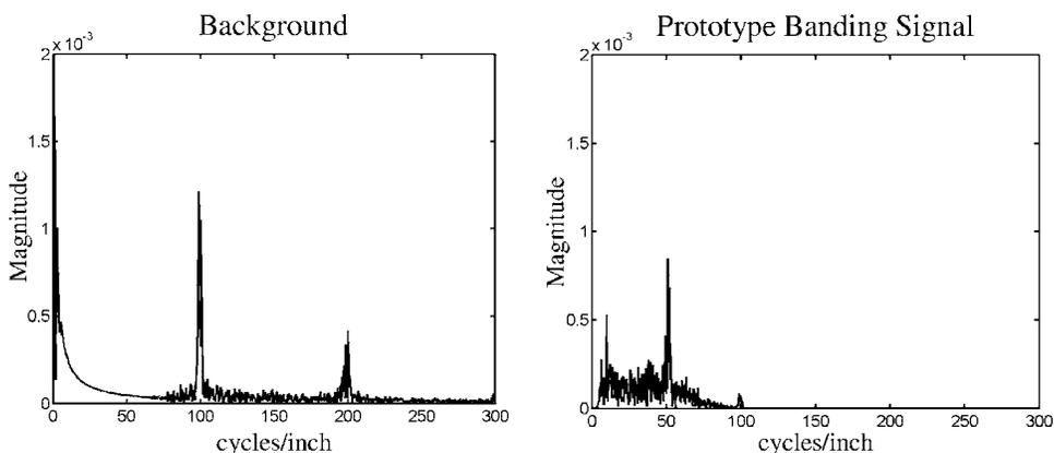
Figure 6. An example of the spectral contents of the background and the prototype banding signal for Printer A.
