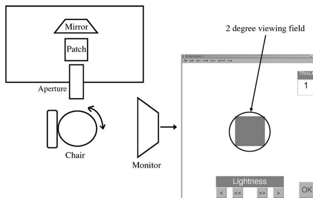
Figure 2. Setup for experiment 1.
