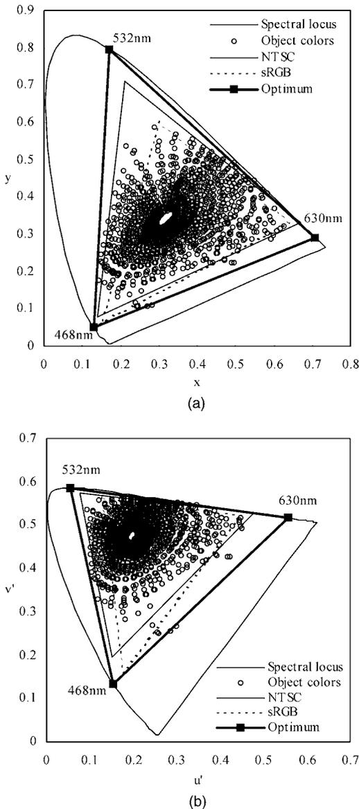
Figure 2. The optimum gamut of real world object colors compared with the standard gamuts on the CIE chromaticity diagram with (a)  $x, y$  coordinates and (b)  $u', v'$  coordinates.
