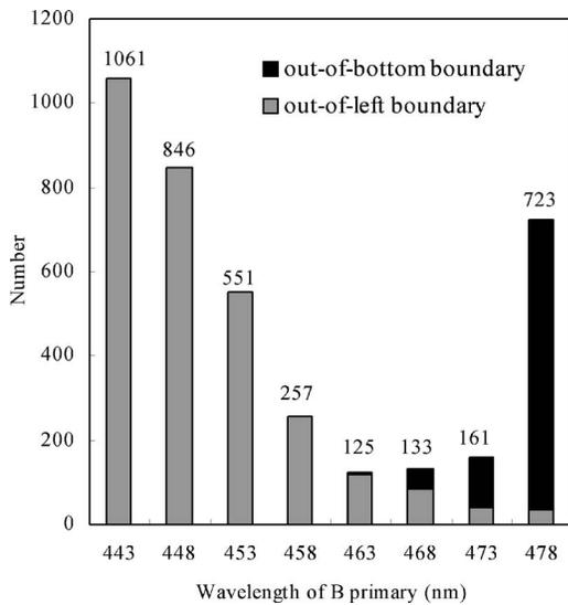
Figure 3. The numbers of out-of-left boundary SOSC data and out-of-bottom boundary SOSC data varies with the shift of B primary.
