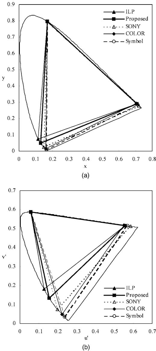
Figure 5. Comparison of four laser display systems' gamut and the optimum gamut on the CIE chromaticity diagram with (a)  $x$ ,  $y$  coordinates and (b)  $u'$ ,  $v'$  coordinates.
