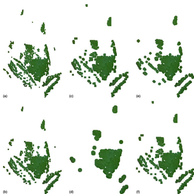
Figure 10. Shows the results of morphological opening with n \times n square structuring elements: (a) 3 \times 3 , (b) 4 \times 4 , (c) 5 \times 5 and disk structuring elements: (d) r=3 , (e) r=4 , (f) r=5 .
